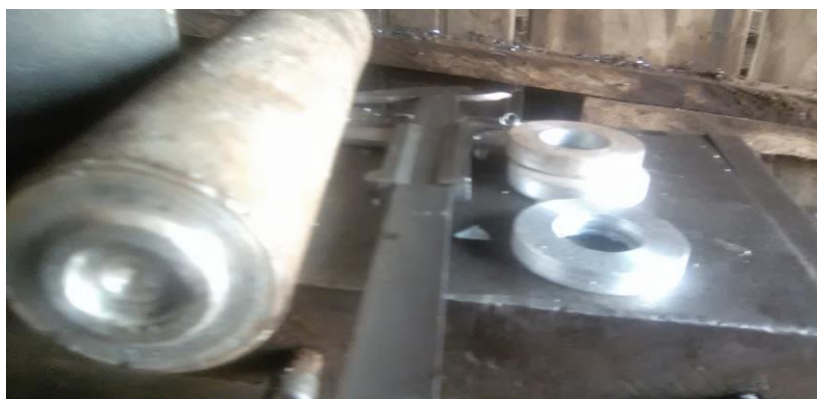
Plate 1: Cast aluminum billet with rings
