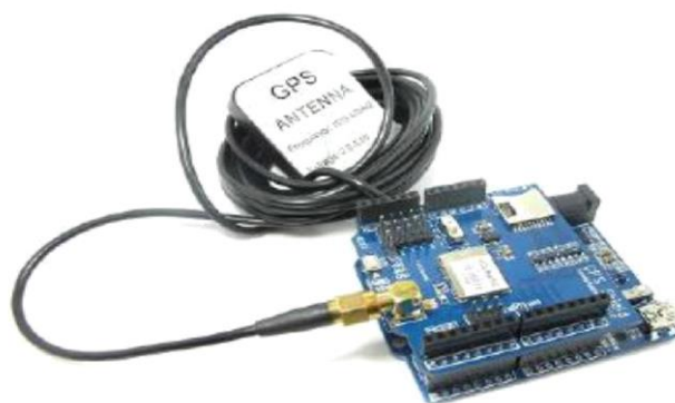
Plate 1: GPS shield and Antenna mounted on Arduino Uno Rev
