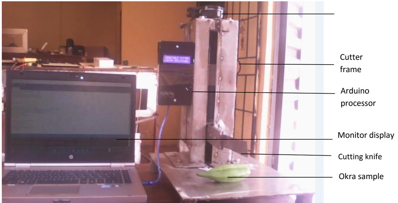
Plate 1.0: Experimental set-up of the cutting mechanism
