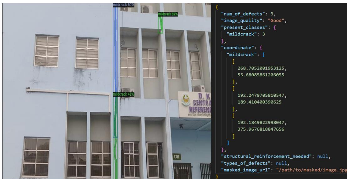
Plate 3: Image of the web application prediction on a mild crack
