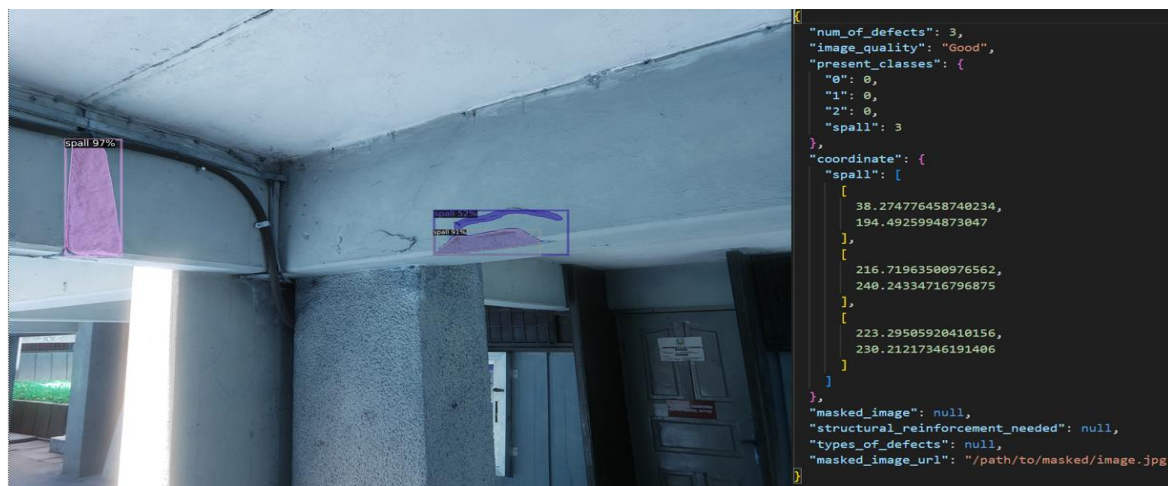
Plate 5: Image of the web application prediction on a mild spall
