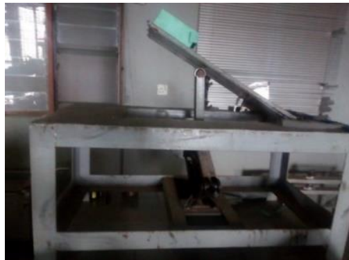
Plate 1: Coefficient of sliding friction determination apparatus
