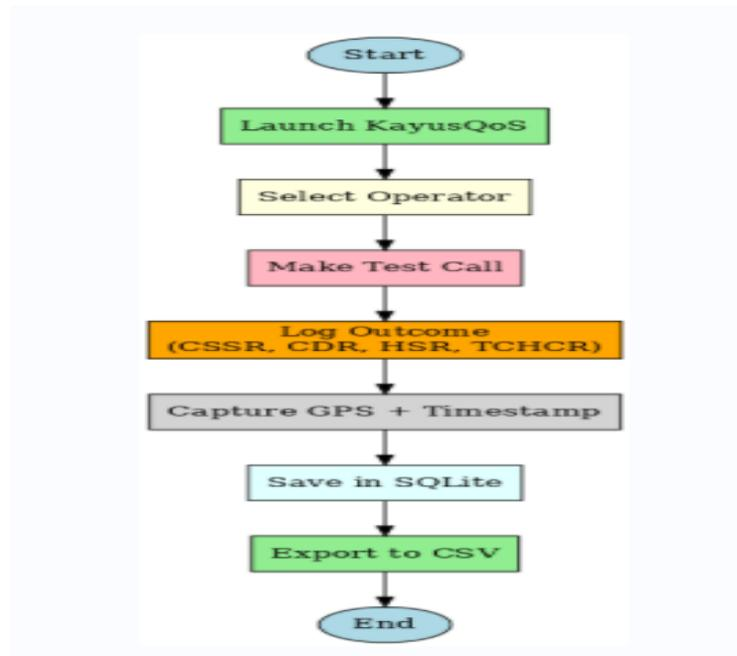
Figure 4: Flowchart of KayusQoS for Capturing Data
