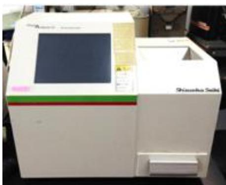
Figure 1. NIR spectrometer, model BR-5000
