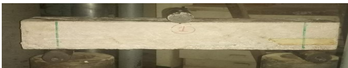
Plate 2: Laboratory Beam Test set up
