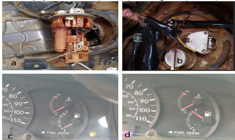
Plate 3: a) Fuel gauge for vehicle b) microcontroller interception of the cable from fuel gauge to dashboard c) vehicle dashboard when fuel level is in reserve d) vehicle dashboard when fuel level is full
