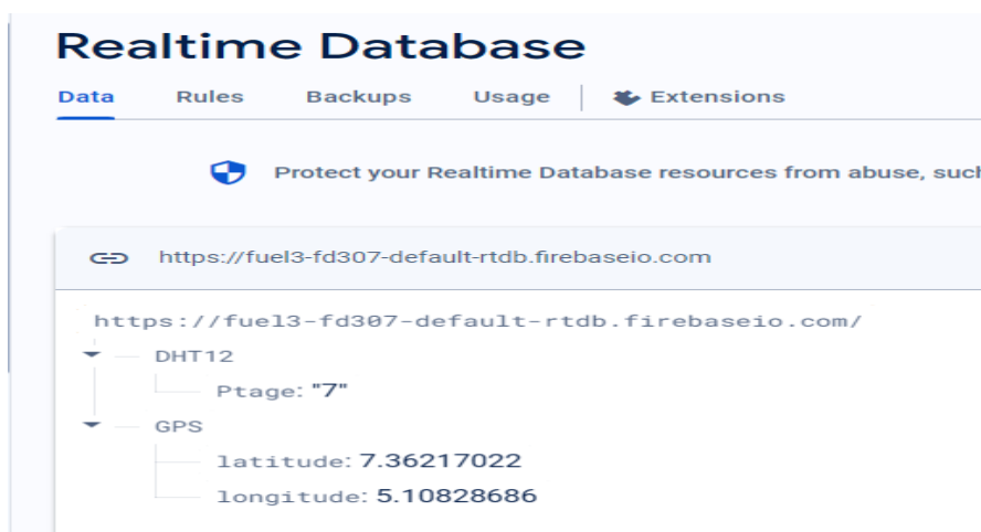
Figure 6: Firebase record of fuel level and GPS coordinates
