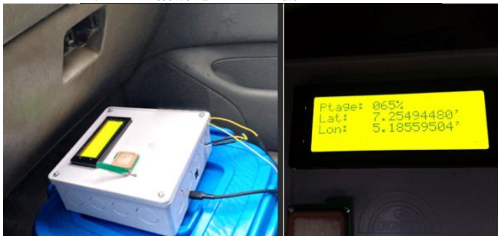
Plate 4: a) Developed device positioned for measurement in the vehicle b) Display showing Ptage: 065%, Lat: 7.25494480, Lon: 5.18559504
