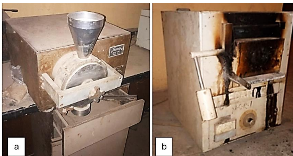
Plate I: a. Milling machine for milling samples, b. Muffle furnace used for SNS carburisation
