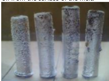
Plate 2: Cylindrical alloy ingot
