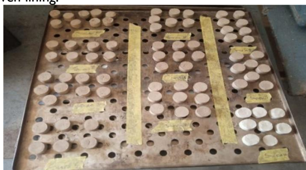
Plate 1: Oven air-dry samples after forming the pellet
