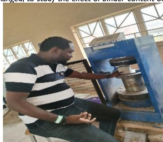
Plate 2: Cube-crushing of concrete samples.
