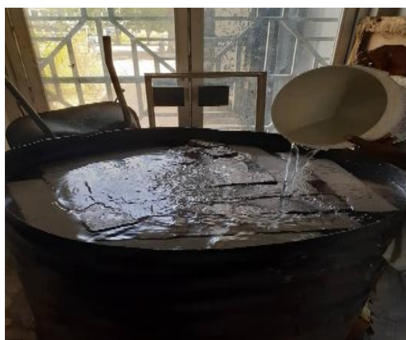
Plate 1: Curing concrete samples.
