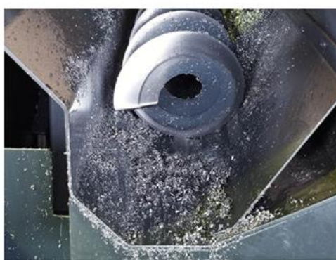
Plate 2: Mild steel Chips collected during Machining
