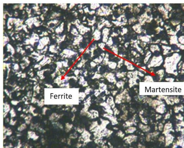
Figure 7: Micrograph of the control sample in as-received condition
