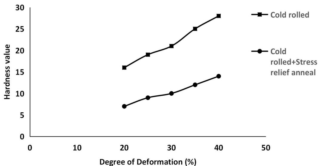
Figure 5: Variation of Hardness with Annealing and Degree of Deformation
