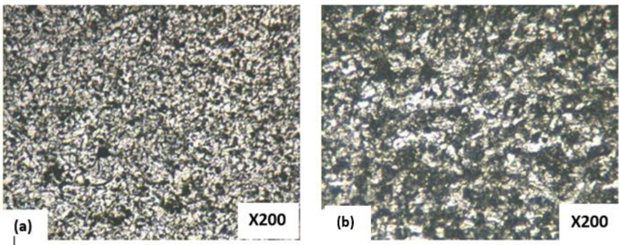
Figure 9: Micrograph of samples at 25% deformation (a) rolled and (b) rolled + stress-relief anneal
