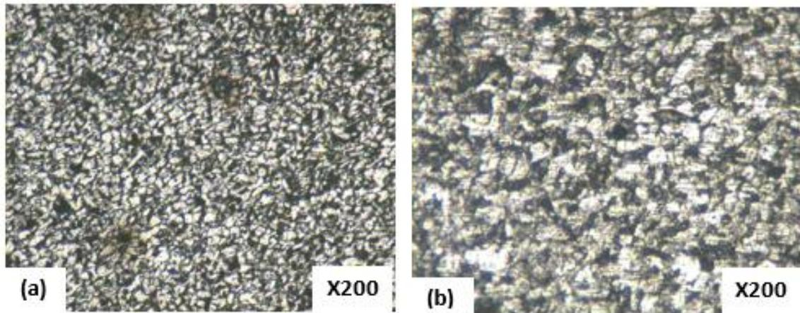
Figure 8: Micrograph of samples at 20% deformation (a) rolled and (b) rolled + stress-relief anneal
