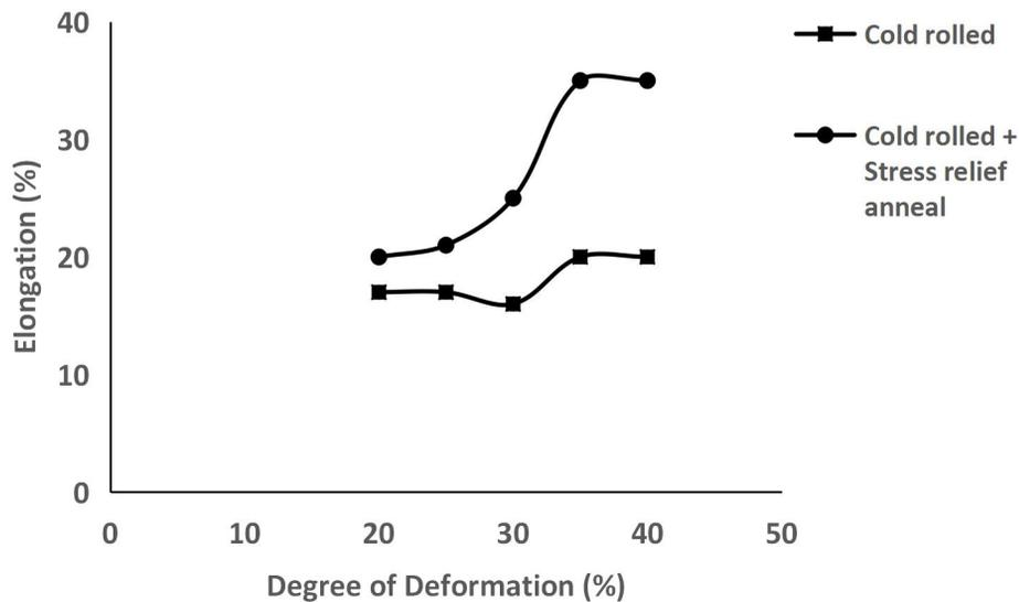
Figure 3: Variation of Elongation with Annealing and Degree of Deformation
