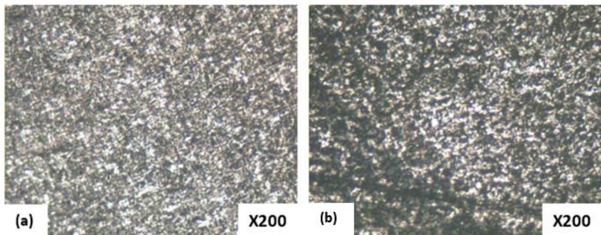
Figure 12: Micrograph of samples at 40% deformation (a) rolled and (b) rolled + stress-relief anneal
