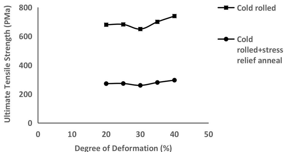
Figure 2: Variation of Ultimate Tensile Strength with Annealing and Degree of Deformation
