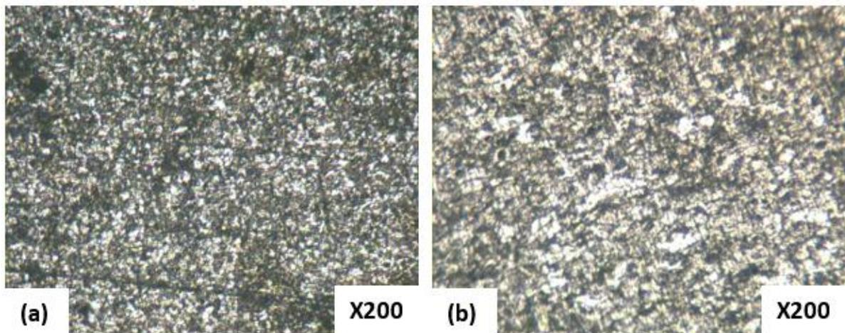
Figure 10: Micrograph of samples at 30% deformation (a) rolled and (b) rolled + stress-relief anneal
