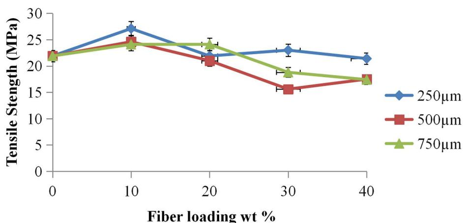
Figure 2: Tensile strength of MHP-HDPE composites at various fiber loadings and sizes
