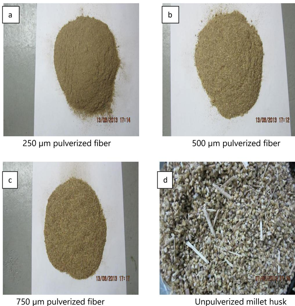
Figure 1: Views of Millet Husks, a) 250  $\mu\text{m}$ , b) 500  $\mu\text{m}$ , c) 750  $\mu\text{m}$  and d) unpulverized)
