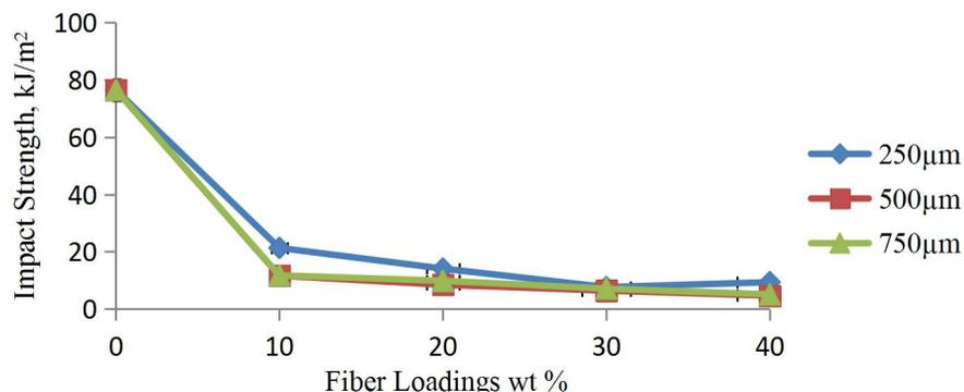
Figure 6: Effects of Fiber Loadings and Sizes on Impact Properties of MHP-HDPE Composites
