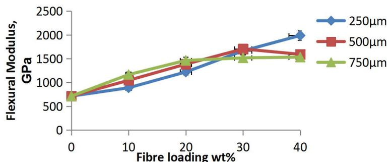
Figure 5: Effects of Fiber Loadings and Sizes on Flexural Modulus of MHP-HDPE Composites
