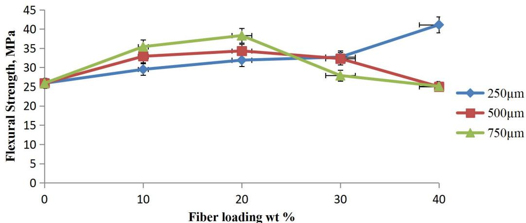
Figure 4: Effects of Fiber Loadings and Sizes on Flexural Strength of MHP-HDPE Composites
