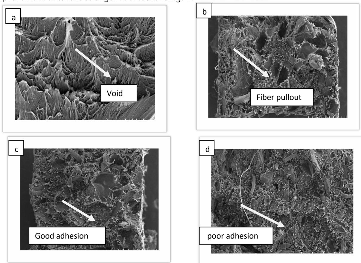
Figure 7: SEM fractomirographs for samples with various fiber loading; (a) 10 % (250  $\mu\text{m}$ ), (b) 30 % (500  $\mu\text{m}$ ), (c) 20 % (750  $\mu\text{m}$ ), and (d) 40 % (750  $\mu\text{m}$ )
