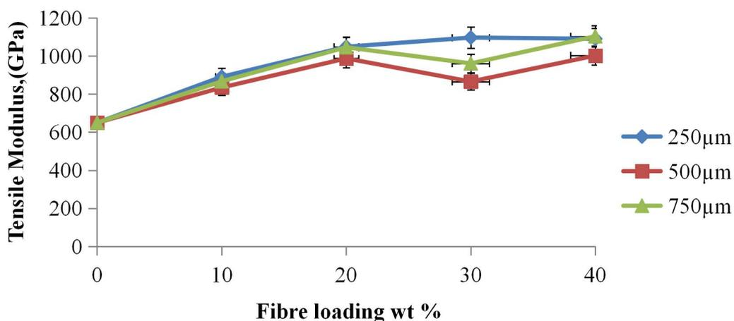
Figure 3: Tensile modulus of MHP–HDPE composites at various fiber loadings and sizes
