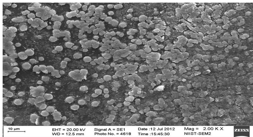
Figure 1: SEM Micrograph for NR/Unmodified kaolin (10 phr)
