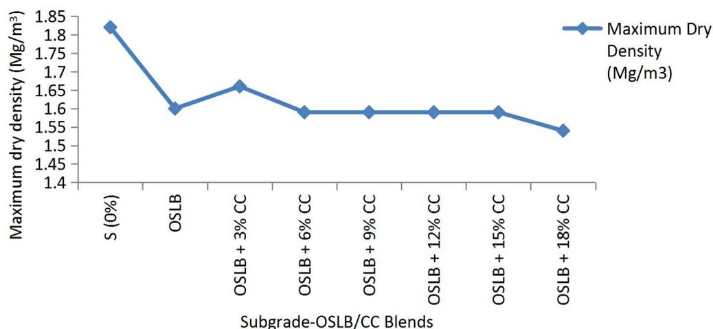
Figure 3: Maximum dry density results of Subgrade-OSLB/CC Blends
