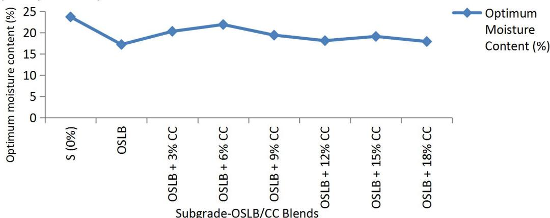
Figure 4: Optimum moisture content of Subgrade-OSLB/CC Blends
