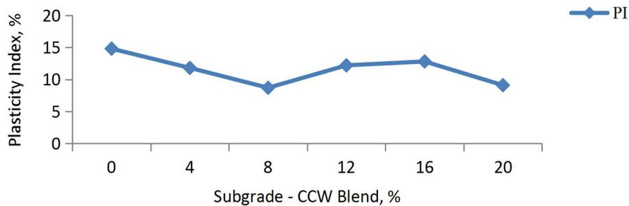
Figure 1: Plasticity Index values of Subgrade - CCW blend
