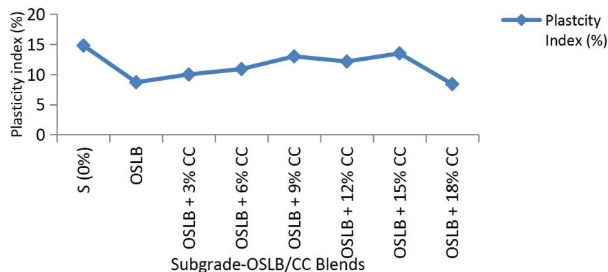
Figure 2: Plasticity index results of Subgrade-OSLB/CC Blends
