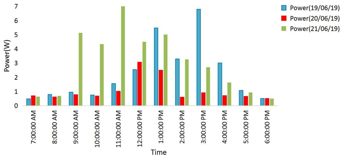
Fig. 19: Solar panel output power against time.
