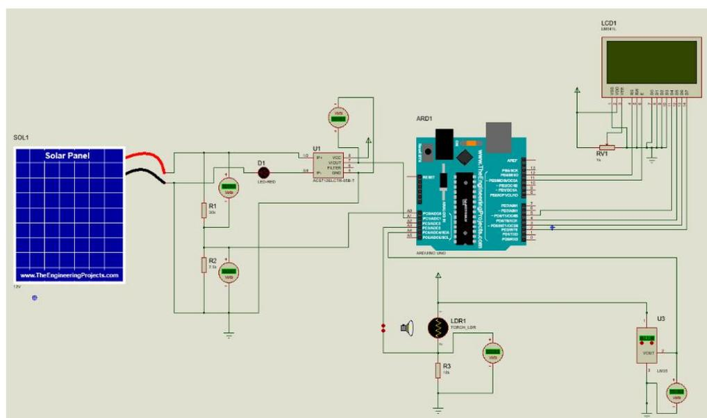
Figure 9: Simulated Solar PV parameter measuring system
