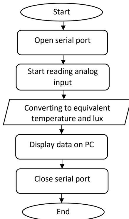
Figure 7: Arduino ADC conversion
