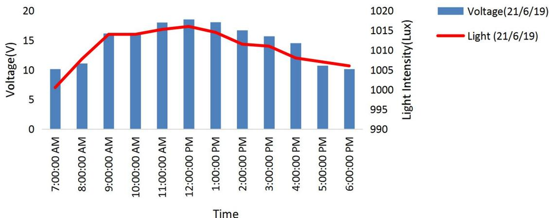
Figure 14: Graph of voltage and light intensity against time for day 3.
