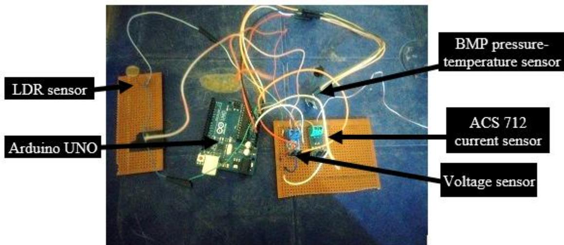
Fig. 10: Constructed solar PV parameter-measuring system
