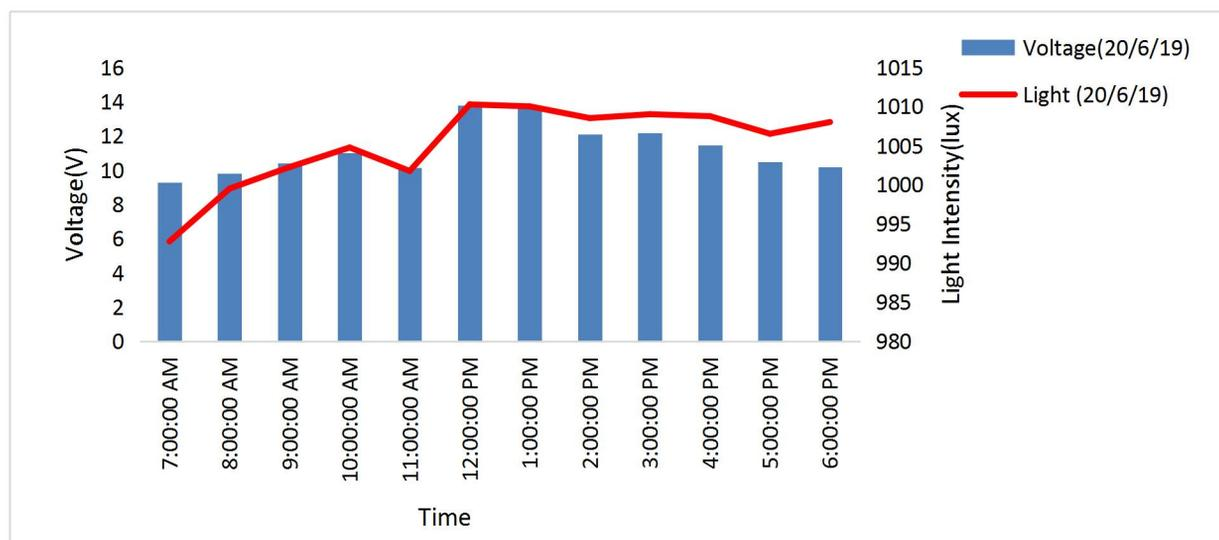
Figure 13: Graph of voltage and light intensity against time for day 2.
