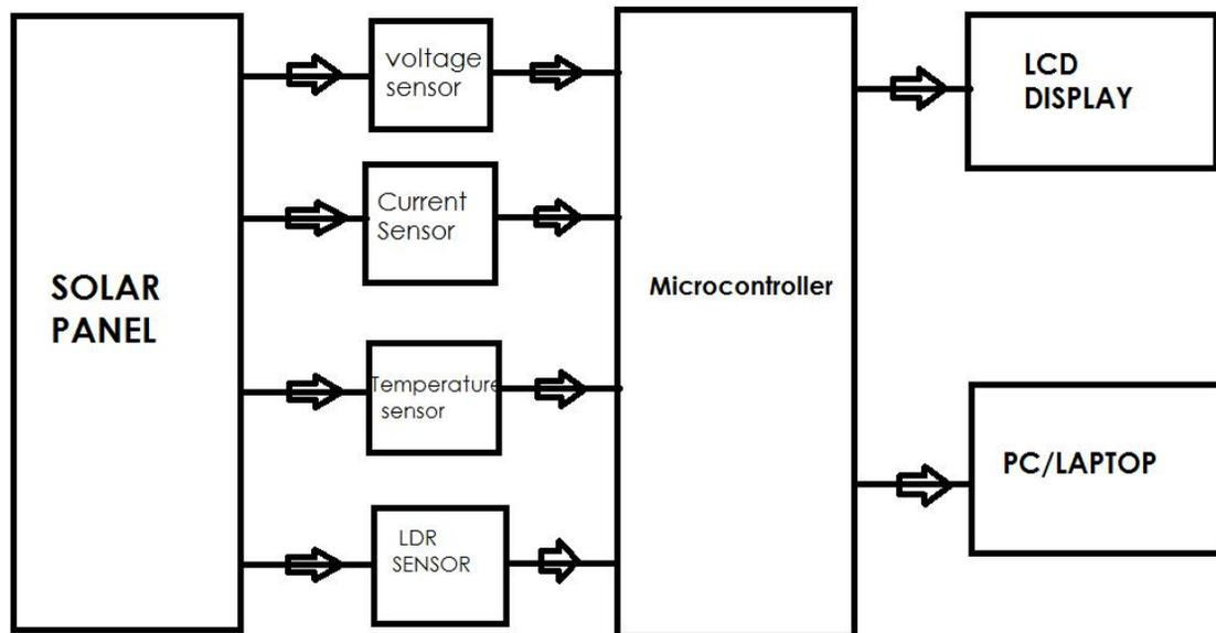
Figure 1: Solar PV parameter-measuring system
