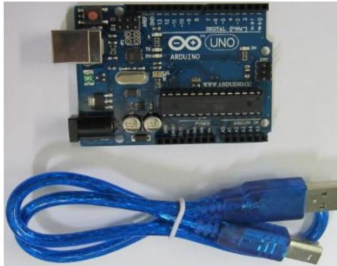
Figure 2: Arduino UNO R3 microprocessor
