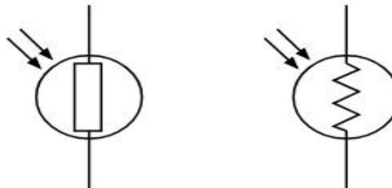
Figure 3: Light dependent resistor
