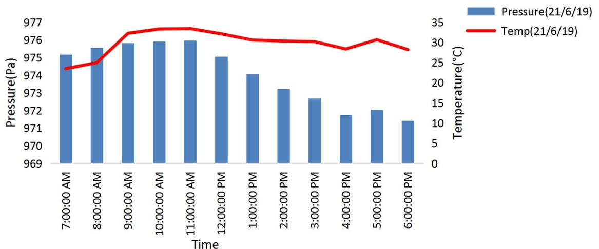
Figure 18: Pressure and temperature against time for day 3
