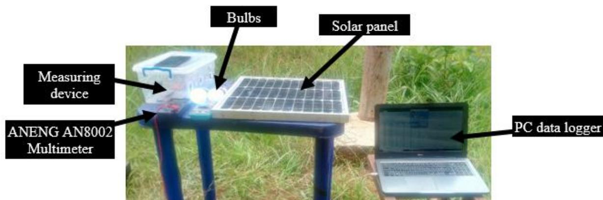
Figure 11: Field testing of measuring system
