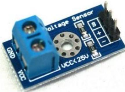
Figure 5: Voltage sensor module
