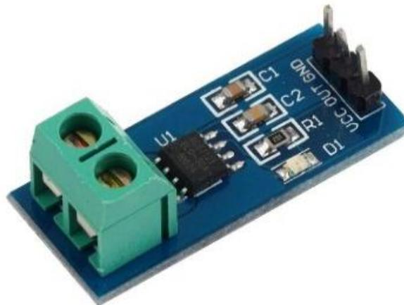
Figure 6: Current sensor module
