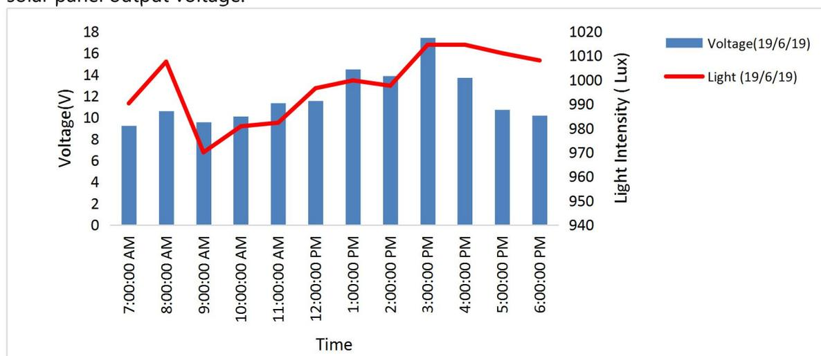
Figure 12: Graph of voltage and light intensity against time for day 1.
