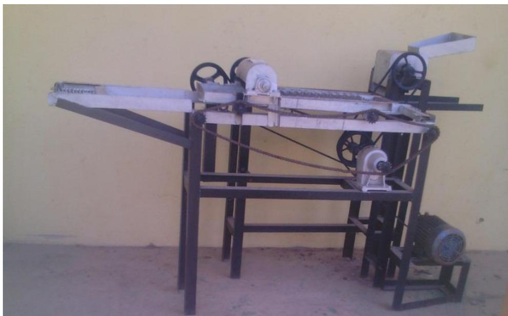
Figure 4. Pictorial View of the Constructed Okra Slicer
