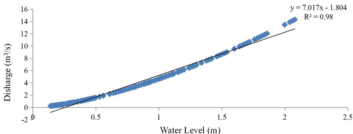
Figure 5. Scattered plot of discharge against water level
