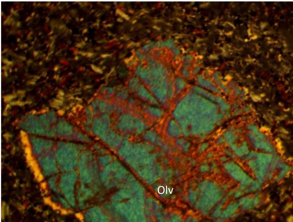
Figure 6: Photomicrograph of basalt showing phenocryst of olivine
