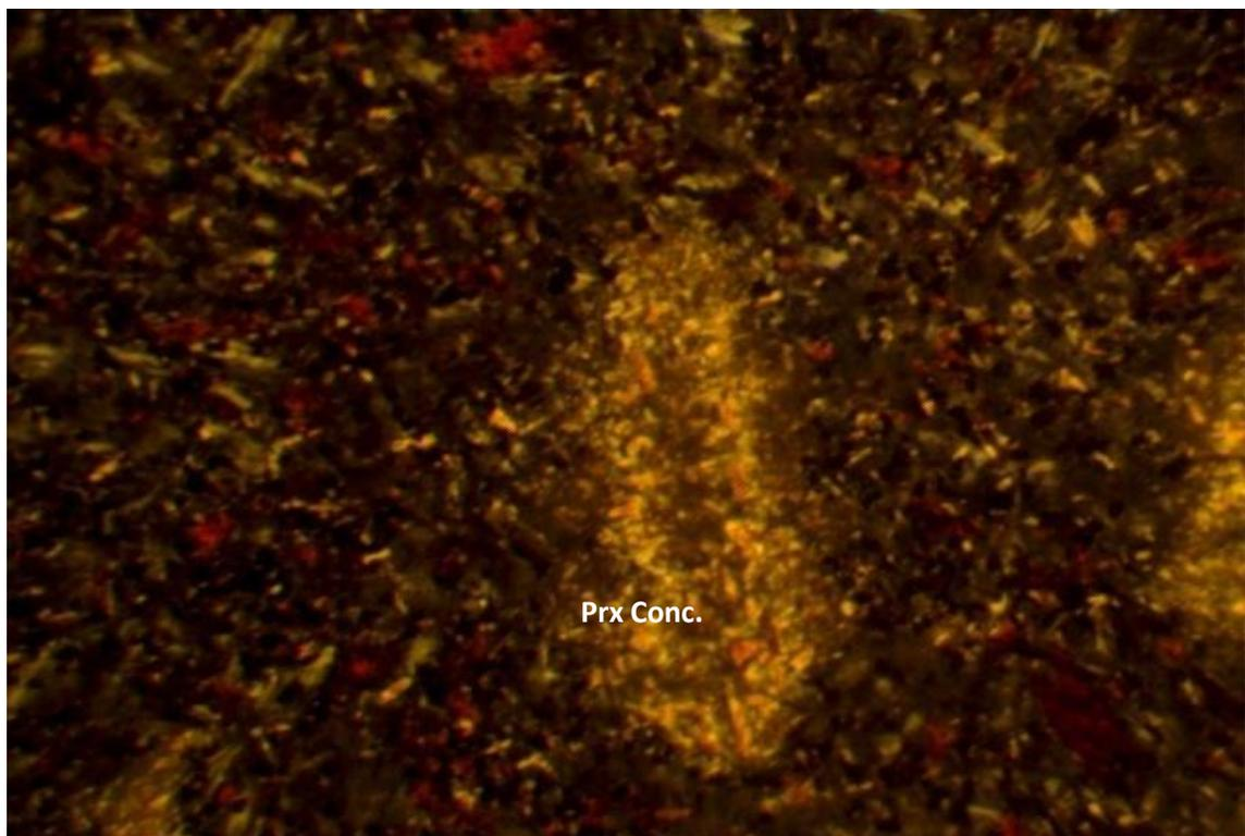
Figure 8: Photomicrograph of basalt showing pyroxene concentration (Prx conc.) in a groundmass of olivine, augite and plagioclase
