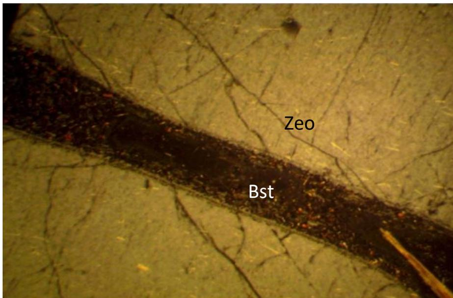
Figure 10: Photomicrograph of basalt showing zeolite being crosscut by groundmass of basalt
