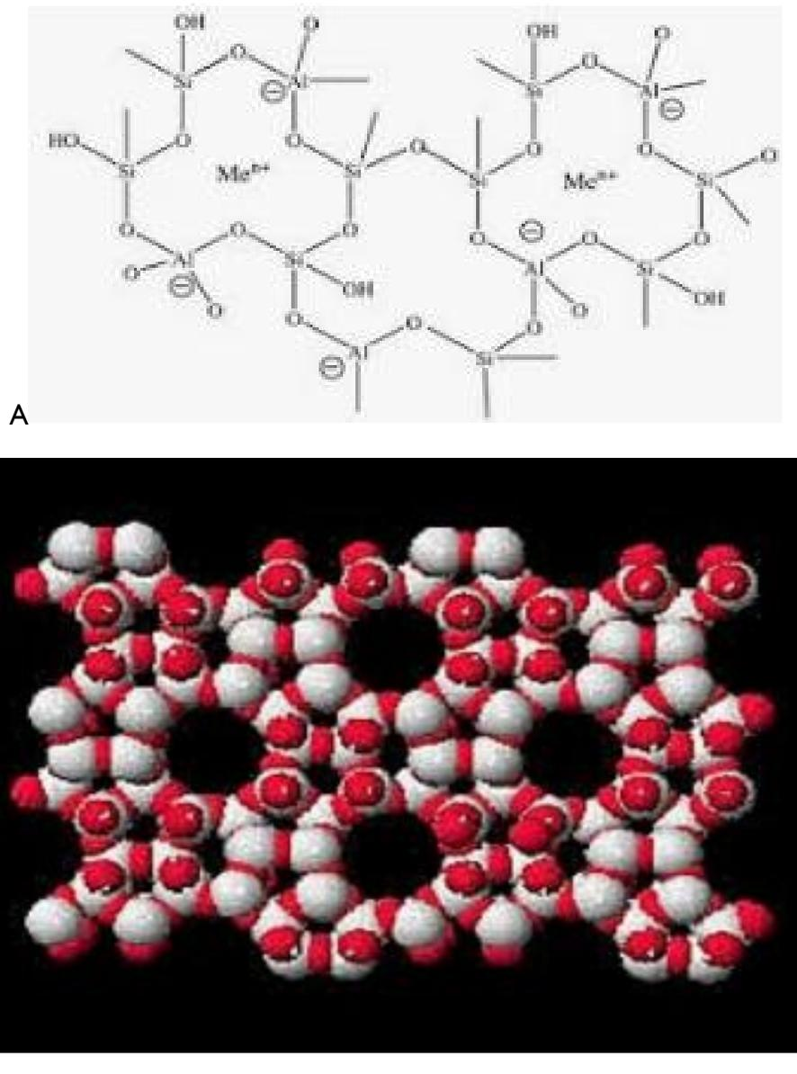
Figure 9: Structures of zeolite, A: framework silicates and B: 3D network of SiO<sub>4</sub> and AlO<sub>4</sub> tetrahedra linked to form channels
