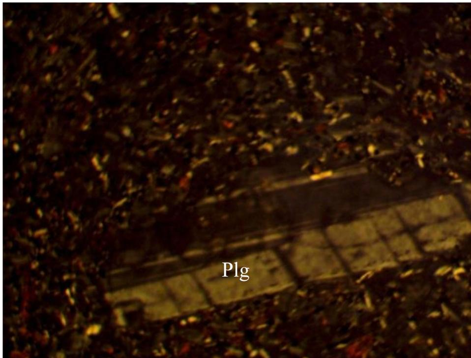
Figure 4: Photomicrograph of basalt showing phenocryst of plagioclase feldspar exhibiting both Carlsbad and albite twinning
