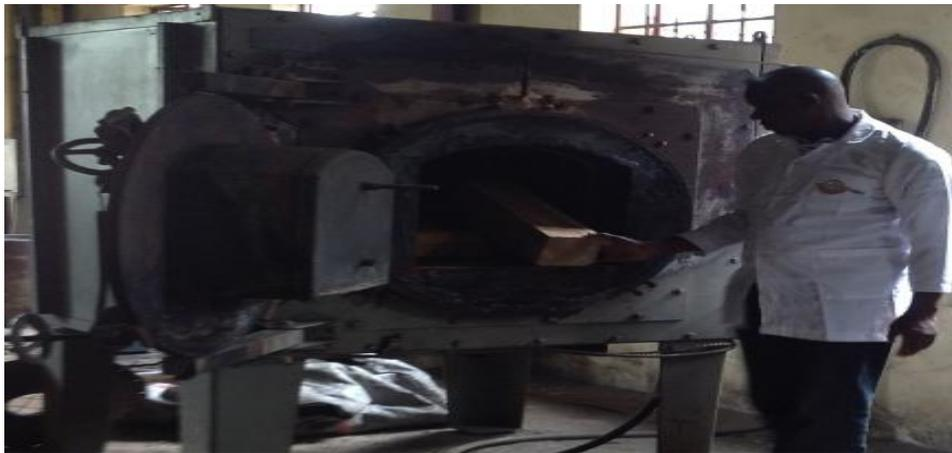
Figure 2: Specimen burning inside furnace
