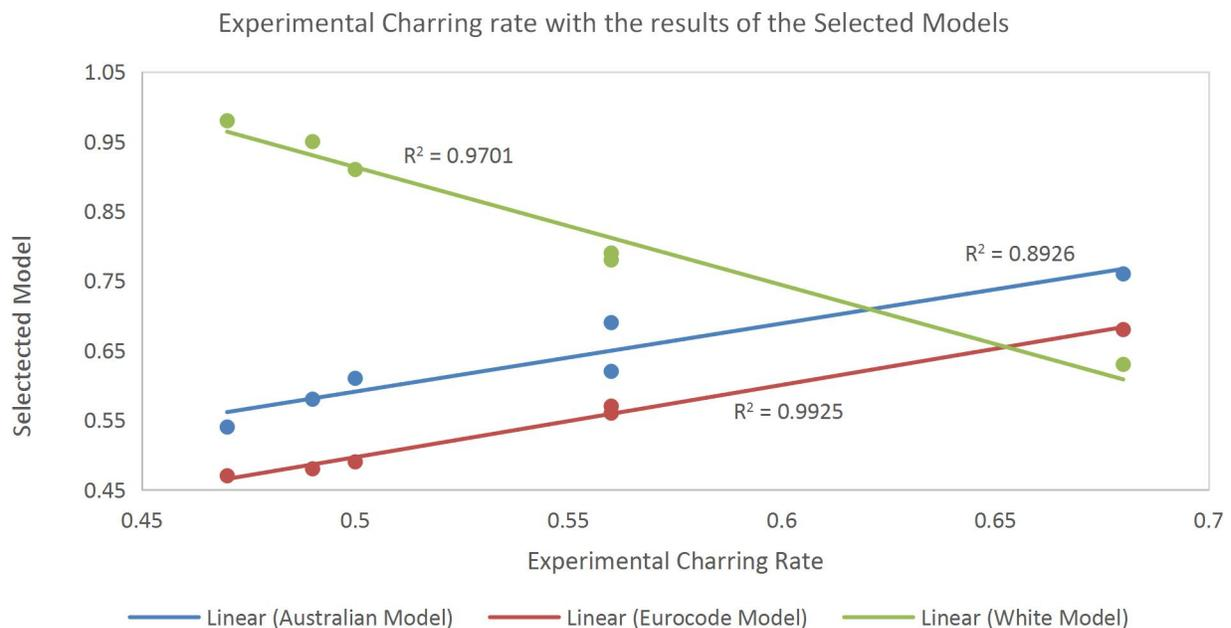
Figure 6: Comparison of Experimental Charring model with the result of Selected Charring models for 15% MC (0-60 minutes) fire exposure temperature at 20°C to 300°C.
