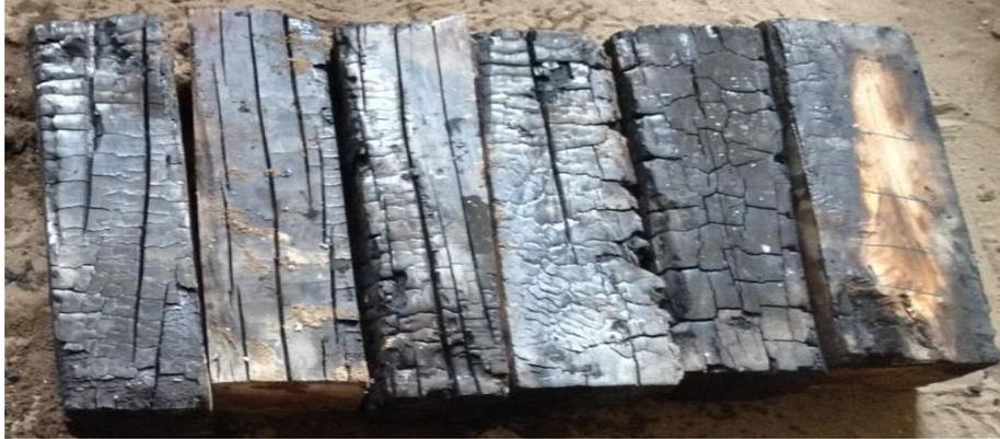
Figure 3: Charred wood after 1-hour fire exposure
