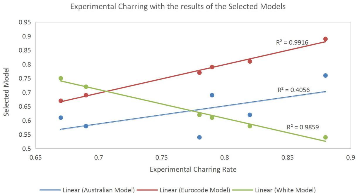
Figure 5: Comparison of Experimental Charring model with the result of Selected Charring models for 15% MC (30 minutes) fire exposure temperature at 230°C to 600°C.
