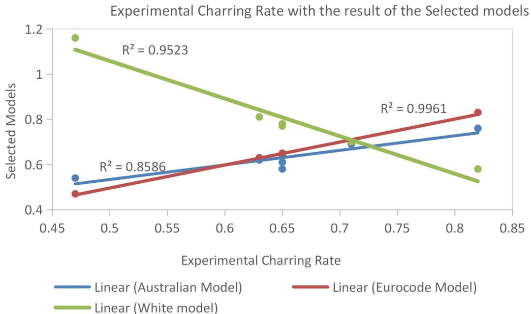
**Figure 4:** Comparison of Experimental Charring model with the result of Selected Charring models for 15% MC (0-30 minutes) fire exposure temperature at 20°C to 230°C.
