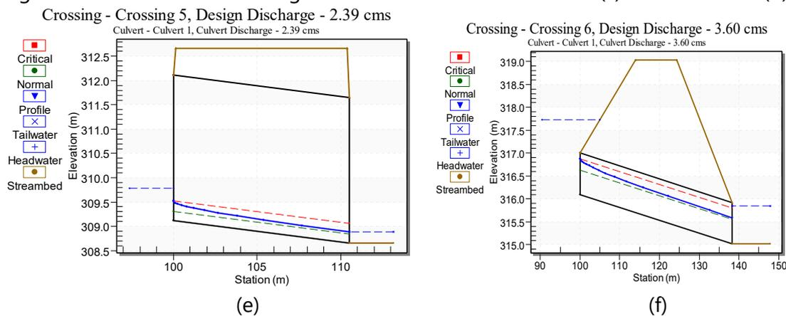
Figure 6: Water Surface Profile generated for Culverts located at (e) Km 7+500 and (f) Km 9+125
