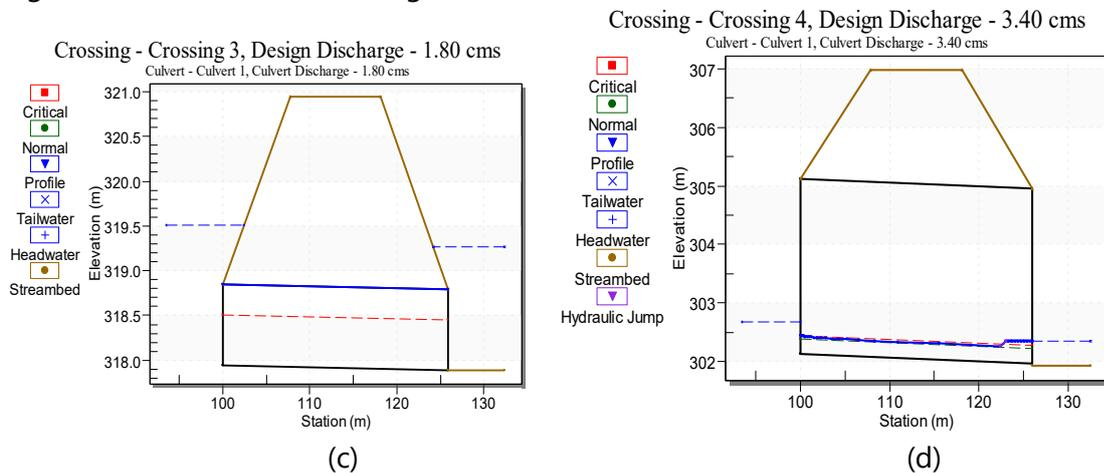
Figure 5: Water Surface Profile generated for Culverts located at (c) Km 3+300 and (d) Km 5+575
