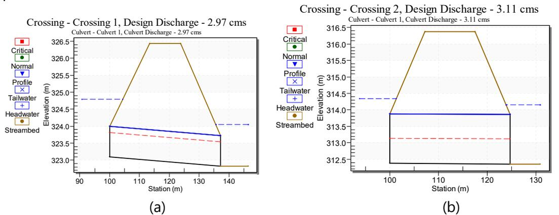
Figure 4: Water Surface Profile generated for Culverts located at (a) Km 1+400 and (b) Km 2+825
