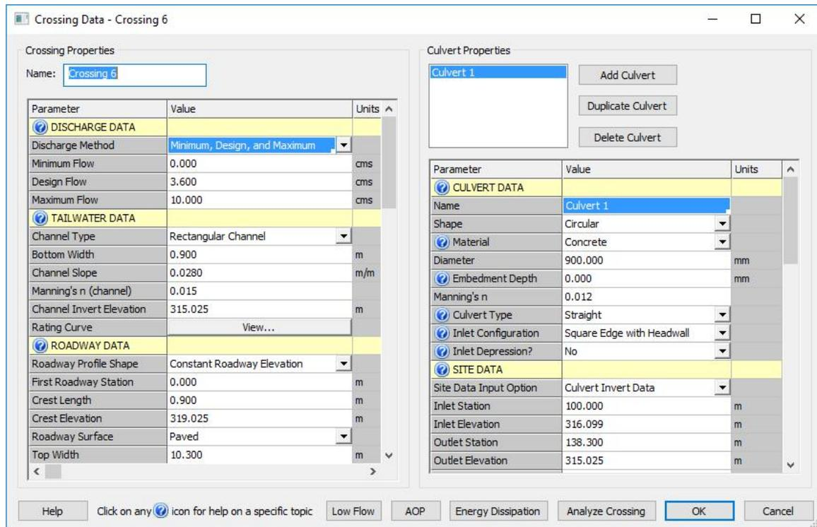
Figure 3: Typical Culvert Crossing Data Window in HY-8 Modelling Tool
