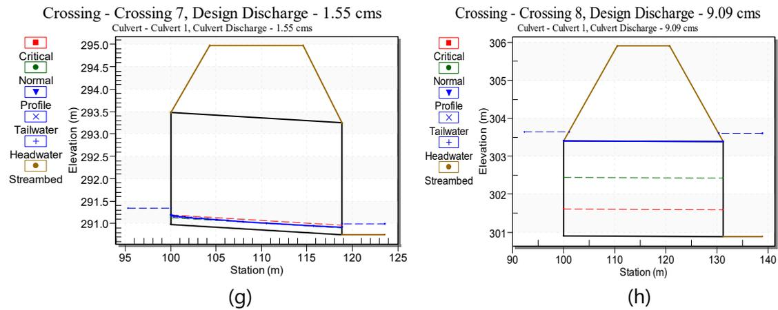
Figure 7: Water Surface Profile for Culverts located at (g) Km10+375 and (h) Km 11+775
