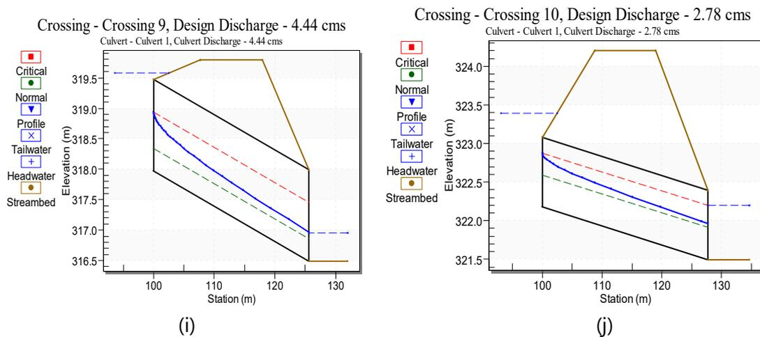
Figure 8: Water Surface Profile for Culverts located at (i) Km12+875 and (j) Km 13+375
