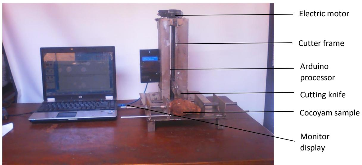
Figure 1.0: Experimental set-up of the cutting mechanism
