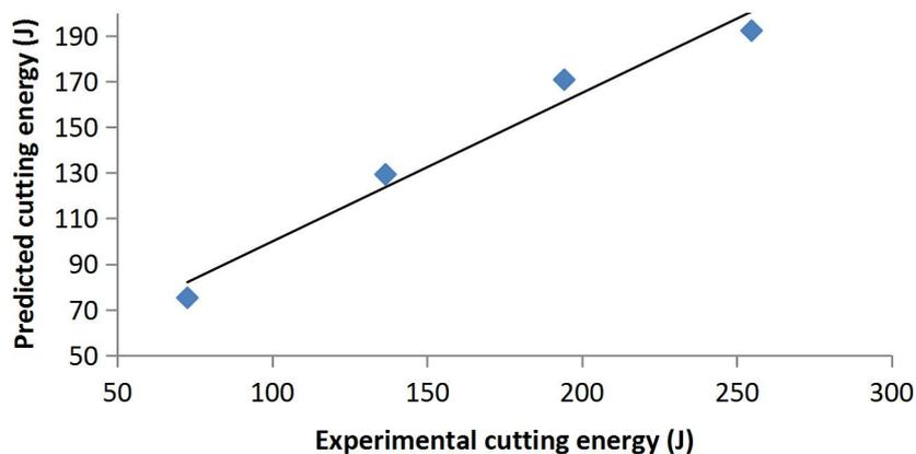
Figure 4: Relationship between experimental and predicted cutting energy. (For summation of component energy equations)
