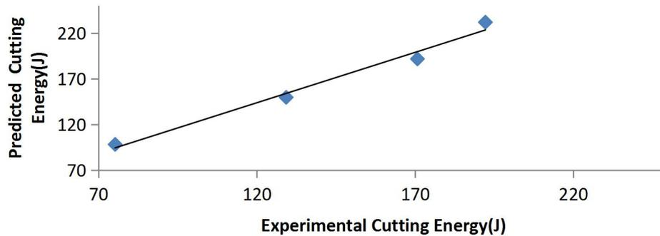
Figure 3: Relationship between experimental and predicted cutting energy (for subtraction of component energy equations)
