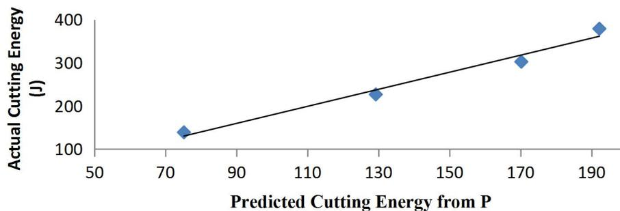
Figure 1: Variation of cutting energy against  $P = \left( \frac{tswH_d}{A} \right)$ , keeping  $Q = \left( \frac{\sigma^2 s^2 H_d}{\phi} \right)$  constant.
