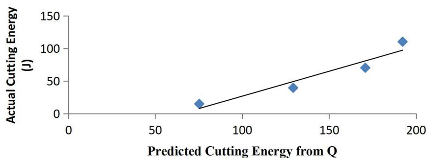
Figure 2: Variation of cutting energy with  $Q = \left( \frac{\sigma^2 s^2 H_d}{\phi} \right)$ , keeping  $P = \left( \frac{tswH_d}{A} \right)$  constant.
