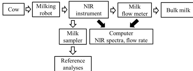
Figure 1. Flow chart of an on-line near-infrared spectroscopic sensing system for determining milk quality in an automatic milking system
