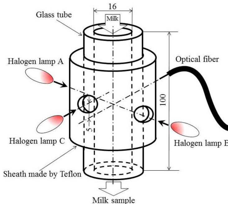
Figure 2. Schematic diagram of the optical system of milk chamber of the NIR spectrum sensor
