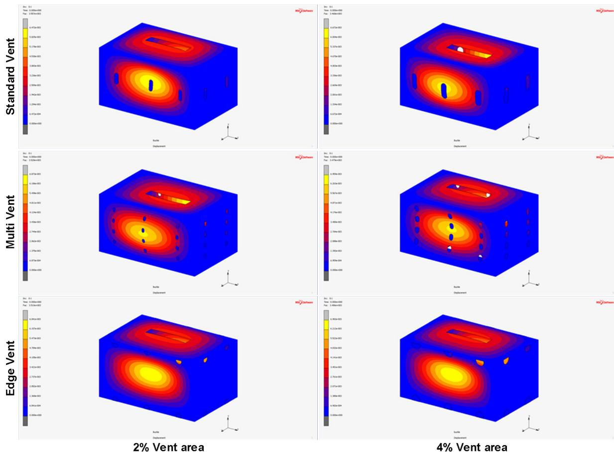
Figure 3. Typical Fringe plots of the buckling of the package designs with B flute board grade.
