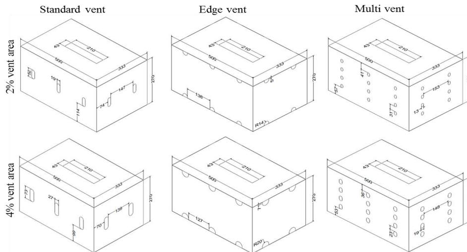
Figure 1. Geometry of the package designs (mm).
