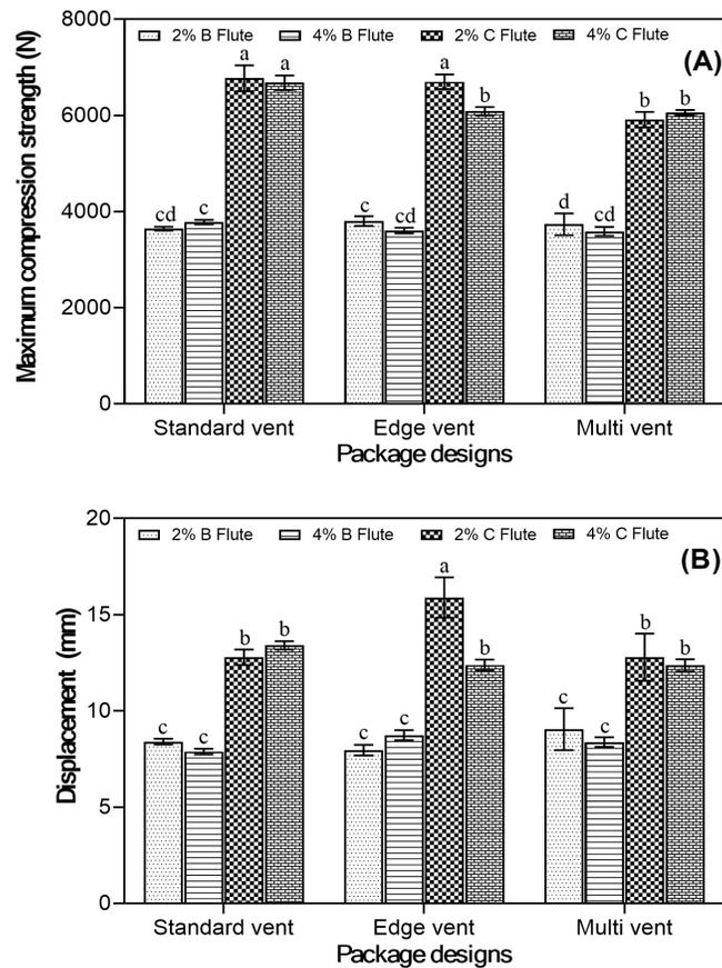
Figure 2. Bar chart showing (A) compression strength and (B) Displacements at maximum compression strength for all the package designs for both B and C flute board at 2% and 4% vent area. The letters on the error bars are used to show the statistical difference. Means with the same letters are not statistically different at  $P \leq 0.05$ .
