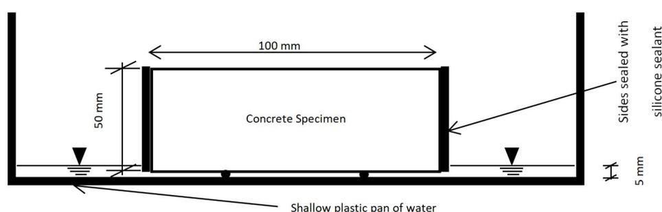
Figure 1: Set up for the measurement of Coefficient of water absorption and sorptivity of Concrete specimens (adaptation from Ganesan et al., 2008).
