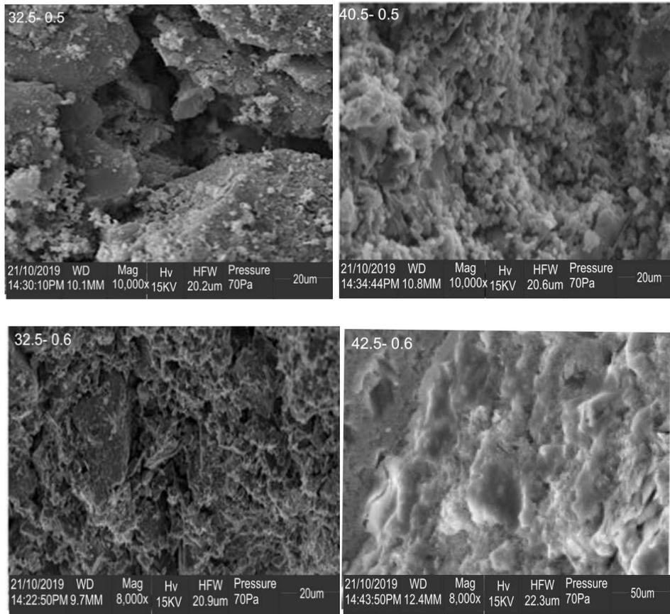
Figure 3: The SEM Micrograph of the Concrete Samples at 28 days of Curing
