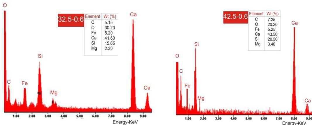
Figure 4: EDX Spectrum of the Concrete samples at 28-day curing
