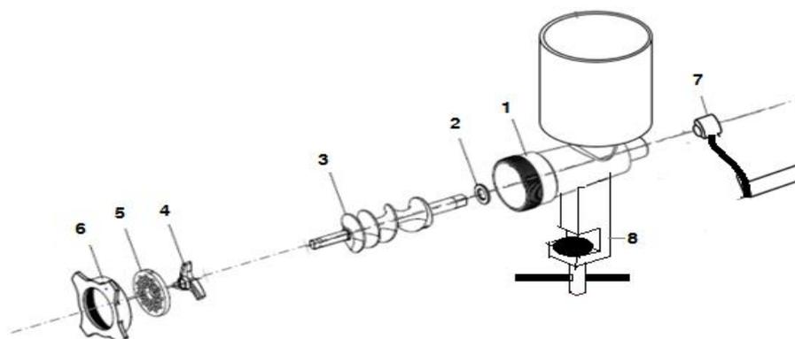
Figure 6: Assembly Sketched of the mincing machine
