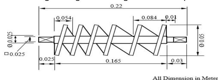
Figure 1: Single start variable pitch worm auger (Shaft)
