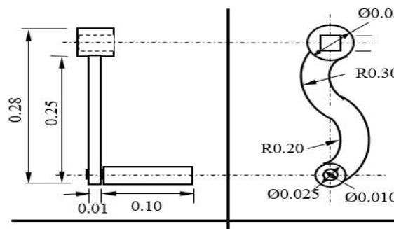
Figure 5: The mincing machine handle
