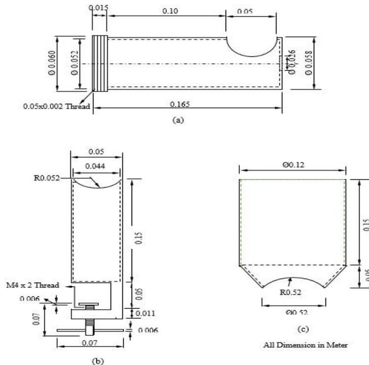
Figure 2: The parts of the mincing head
