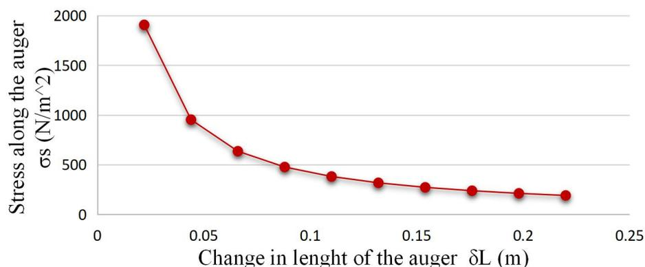
Figure 7: Stress distribution along the length of the auger
