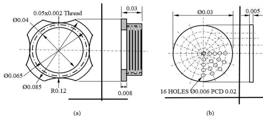
Figure 3: Mincing head cover and perforated plate
