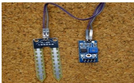
Figure 3: Soil moisture sensor
