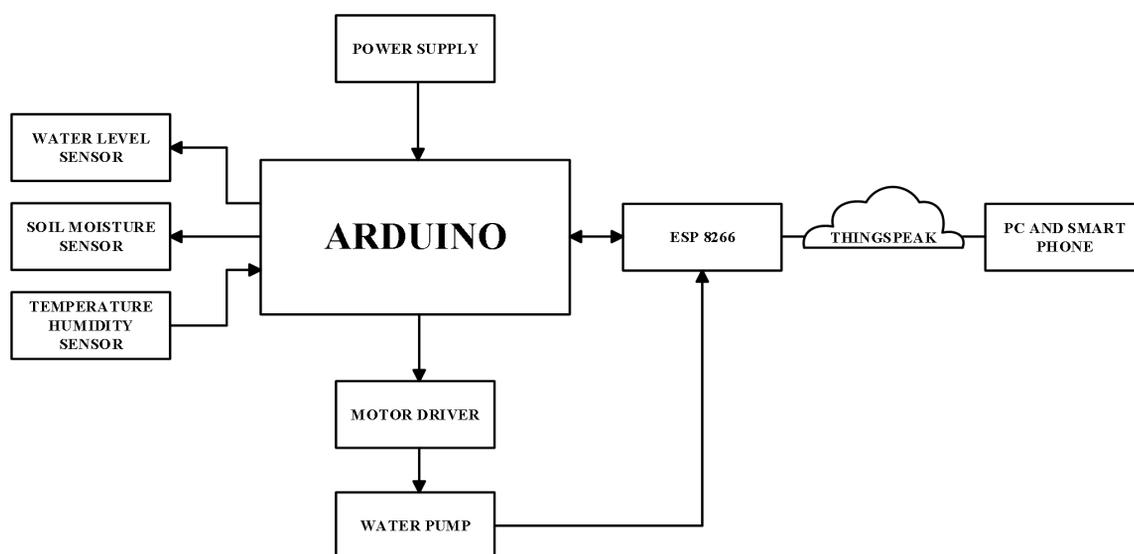
Figure 1: Block diagram of an IoT based Irrigation System
