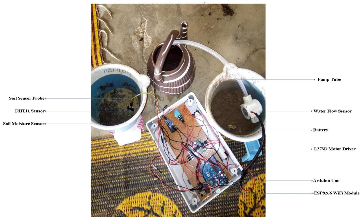
Figure 11: Prototype system
