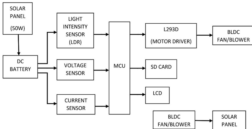
Figure 3: Block diagram of the PV system incorporated with a soiling mitigation technique
