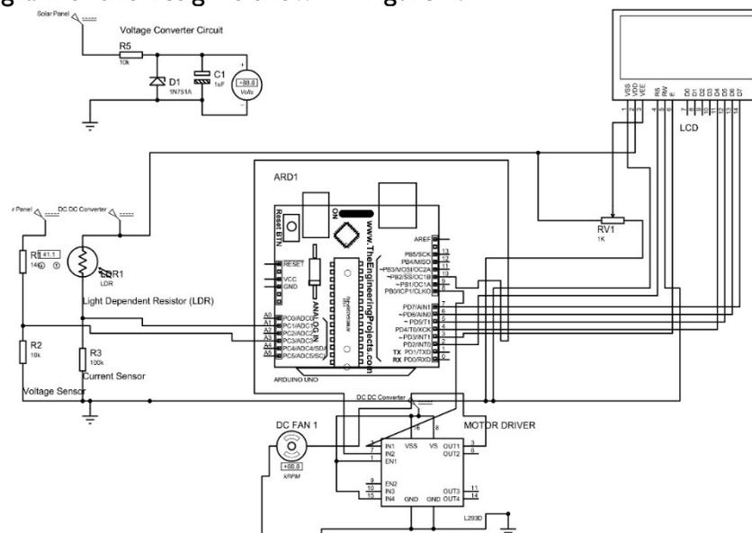
Figure 4: System circuit diagram designed using proteus
