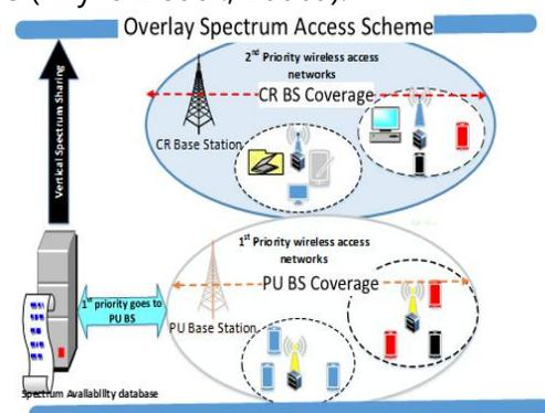
Figure 3: Spectrum Overlay Dynamic Spectrum Scheme (Mustapha, 2016)
