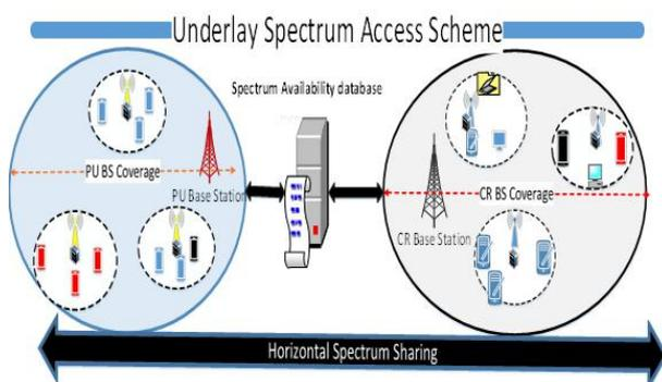
Figure 2: Spectrum Underlay Dynamic Spectrum Scheme
