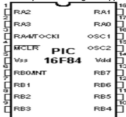
Figure 2: Pin assignment of PIC 16F84A
