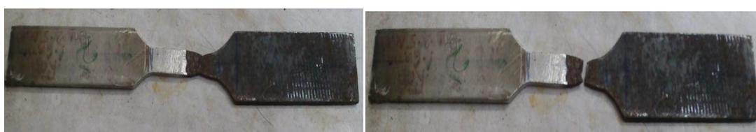
Figure 2: Mild steel/stainless steel dissimilar welded Joint before and after tensile test
