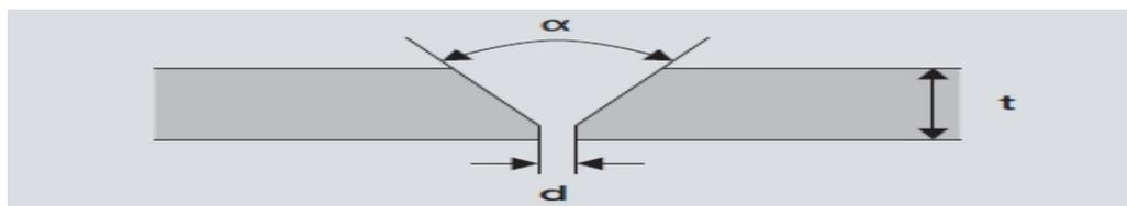
Figure 1: Schematic Representation of the Welded Joint
