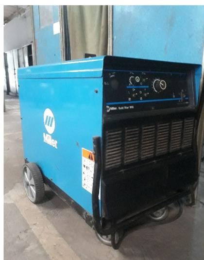
Figure 4a: GTAW Welding Machine
