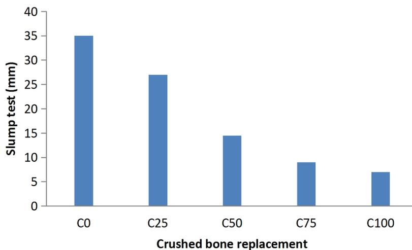
Figure 2: Variation of slump values with crushed bone replacement
