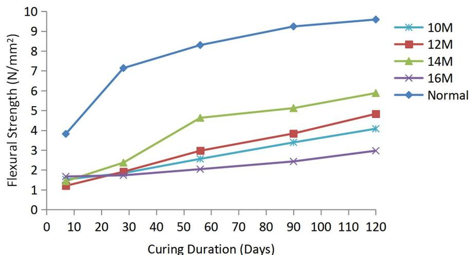
Figure 6: Flexural strength of AACSAM and control
