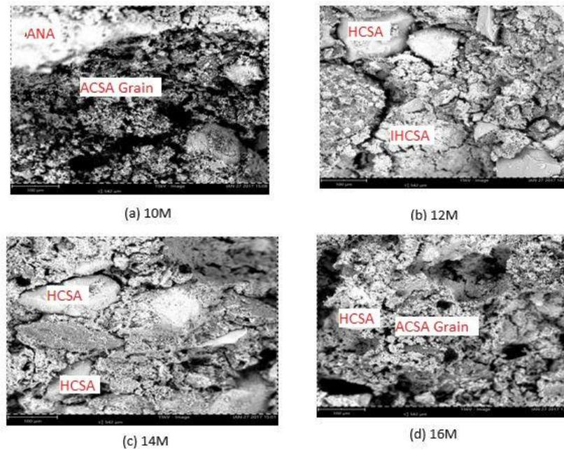
Figure 7: SEM images of AACSAM at 28 days of hydration with different NaOH concentrations. ANA: Anhydrous NaOH, ACSA: Anhydrous CSA, HCSA: Hydrated CSA; IHCSA: Incomplete Hydrated CSA
