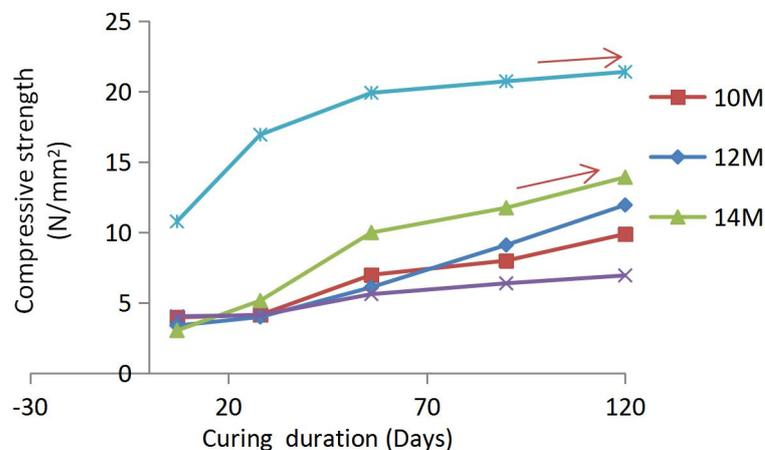
Figure 5: Compressive strength of AACSAM and control
