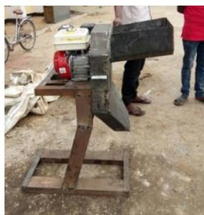
Plate 1: Photograph of the hammer mill
