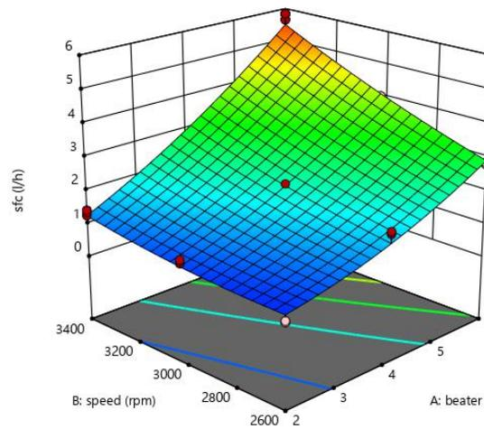
Figure 4: Effects of hammer speed and number of beaters on sfc for percentage maize milled
