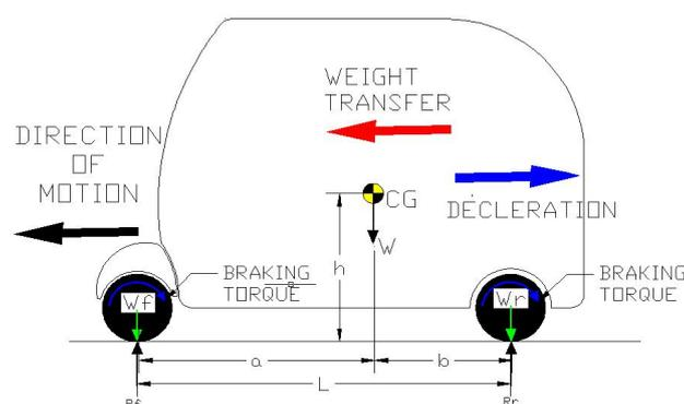
Figure 8: Weight Transfer (Developed from; Giri (2010)).
