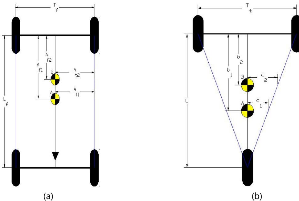
Figure 4: The Effects of Loading. (a). Four Wheeled Vehicle, (b) Three Wheeled Vehicle. (Adapted from; Kenneth et al. 1996)
