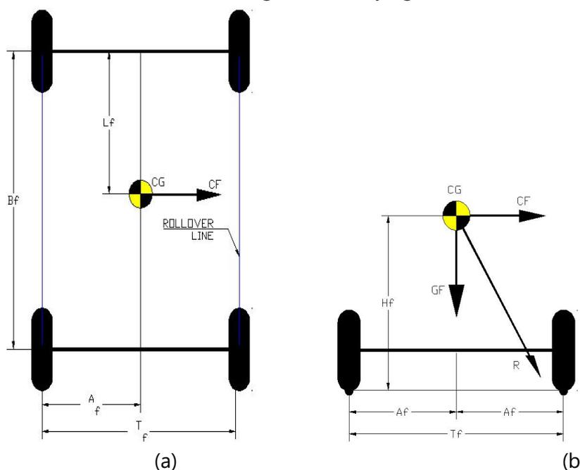
Figure 2: Position of Centre of Gravity (Developed from; (Palash et al. 2014). (a) Top view of Four Wheeled Vehicle. (b) Rear view of Four wheeled Vehicle.
