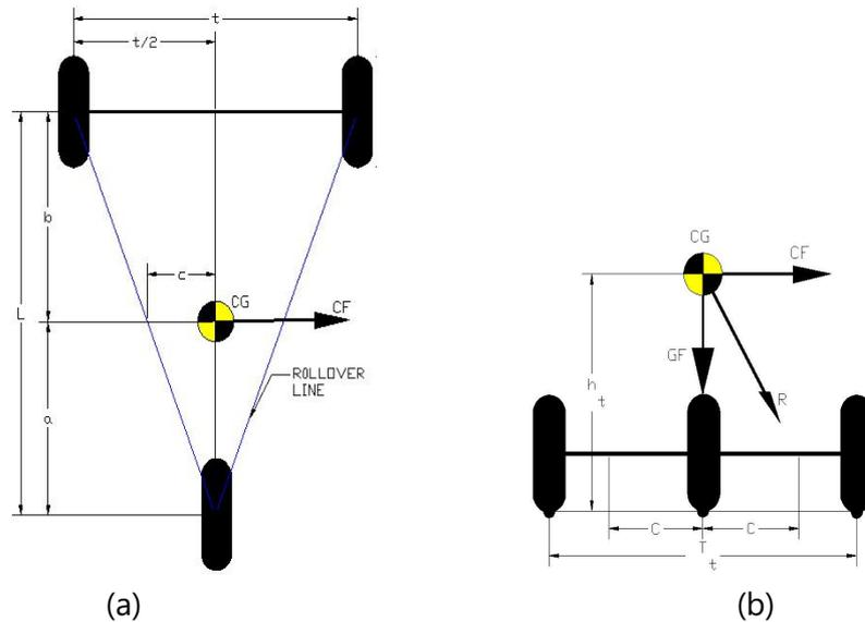
Figure 3: Position of Centre of Gravity (Developed from Palash et al., 2014). (a) Top view of Three Wheeled Vehicle. (b). Rear View of Three Wheeled Vehicle.
