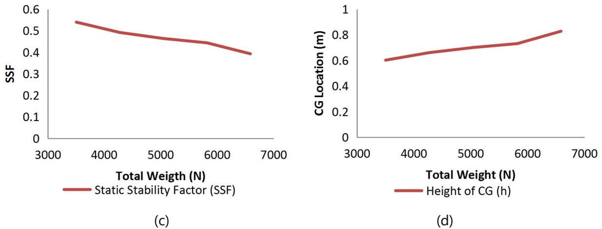
Figure 7: (a) CG from Front and Rear Wheel (b). CG from Roll Overline. (c) Static Stability Factor (SSF). (d) Height of CG (h).
