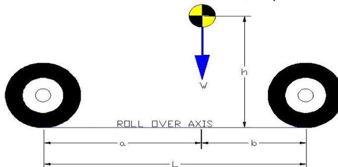
Figure 6: Side-view of the vehicle showing the vertical force (weight).
