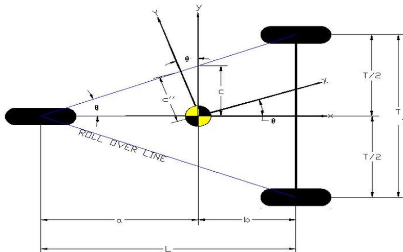
Figure 5: Lateral distance from CG to rollover axis (Adapted from Azadeh, 2014)
