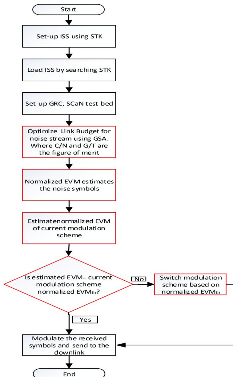
Figure 1: Flowchart of the Developed Improved Developed Improved adaptive coding and modulation scheme
