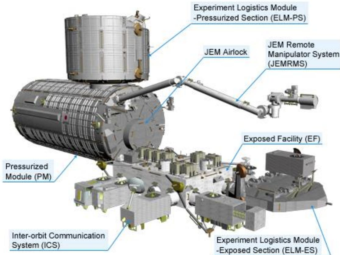
Figure 1 Kibo Configuration Showing Its Segments (JAXA, 2007b)
