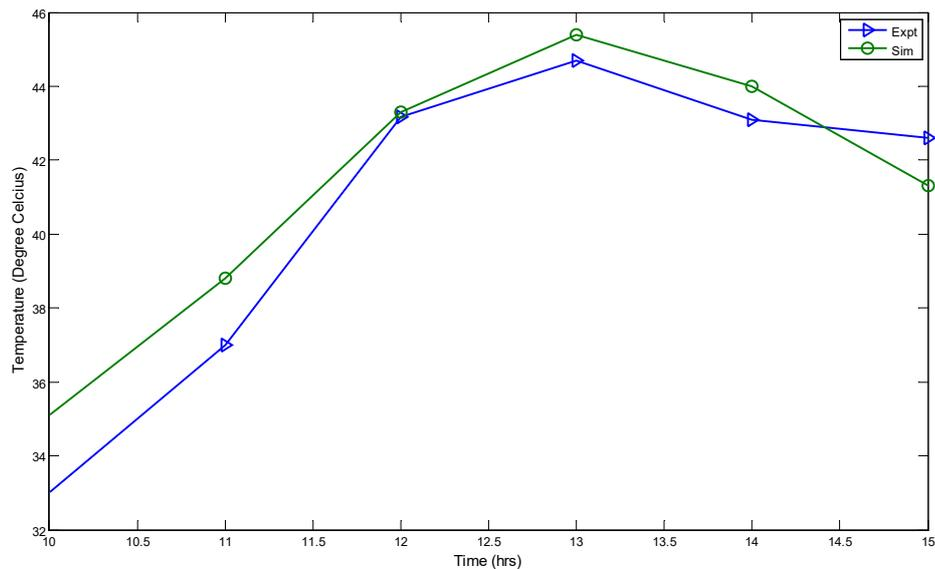
Figure 7: Comparison of experimental and simulated hourly average drying temperature for all trays recorded with the predicted values (0.036 kg/s)
