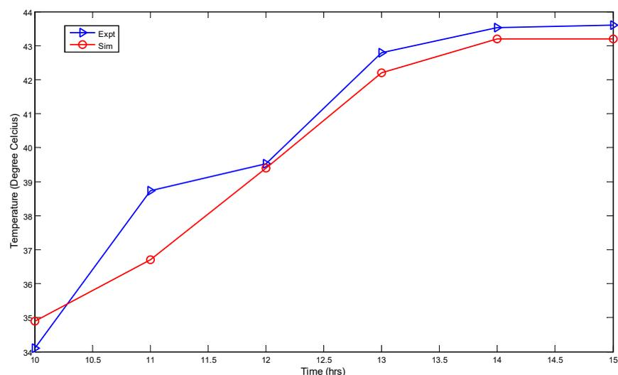
Figure 3: Comparison of experimental and simulated hourly average drying temperature for all trays recorded with the predicted values (0.026 kg/s)
