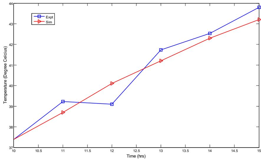
Figure 4: Comparison of experimental and simulated hourly average drying temperature for all trays recorded with the predicted values (0.033 kg/s)
