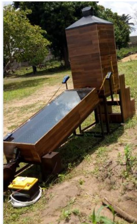
Figure 1: Complete assembly of the experimental rig
