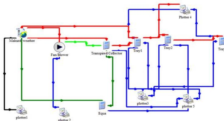
Figure 2: Structure of Transpired Solar Drying System Schematic Model in TRNSYS
