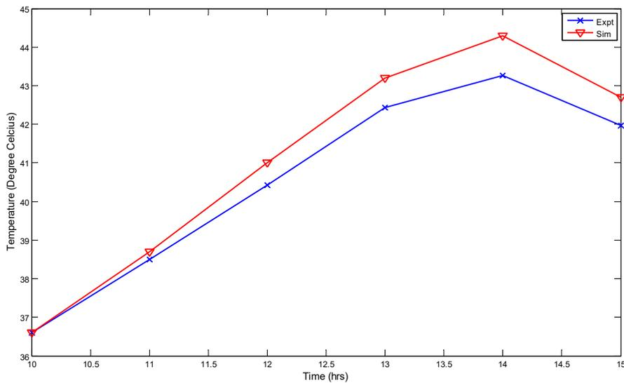
Figure 5: Comparison of experimental and simulated hourly average drying temperature for all trays recorded with the predicted values (0.034 kg/s)
