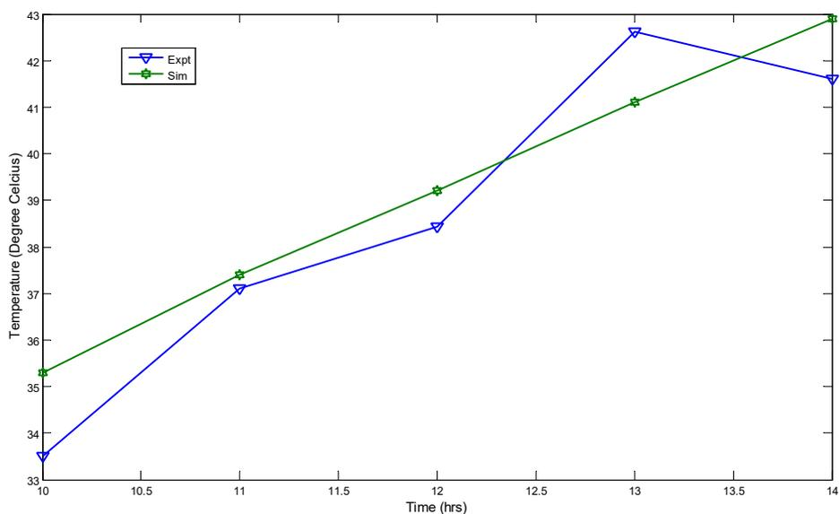
Figure 6: Comparison of experimental and simulated hourly average drying temperature for all trays recorded with the predicted values (0.035 kg/s)
