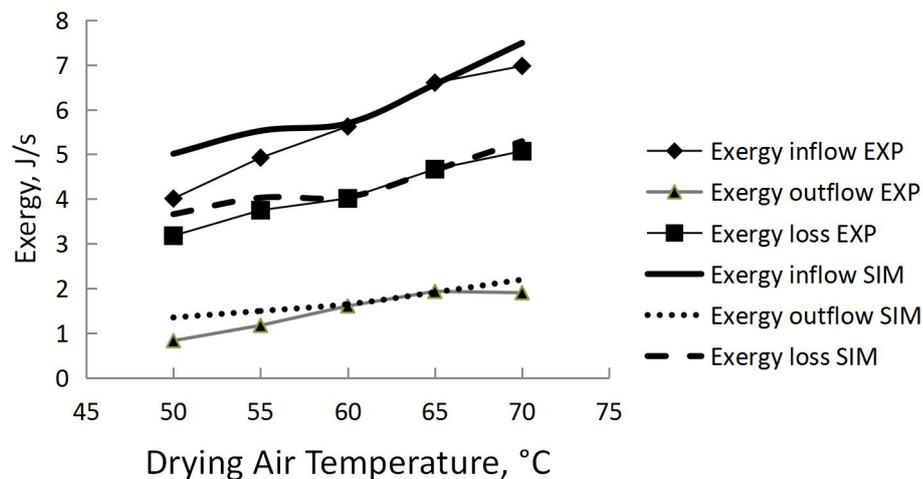
Figure 4: Effect of drying temperature on the exergy inflow, outflow and loss.
