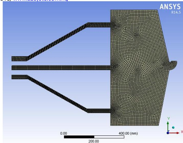
Figure 2: Discretization of the 2D model of the CSRTC Dryer
