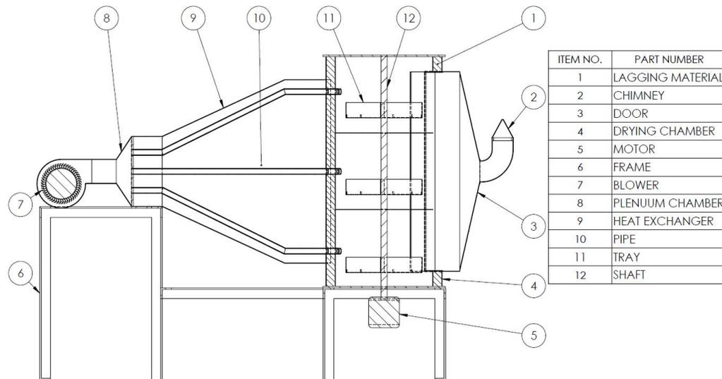
Figure 1: Schematic diagram and part list of the CSRTC tray dryer.
