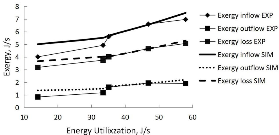
Figure 5: Effect of energy utilization (EU) on the exergy inflow, outflow and loss.
