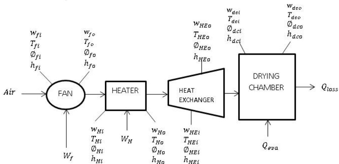
Figure 3: The mass-energy model for the drying experiment in respect to the components
