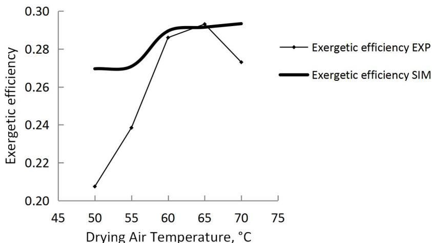
Figure 6: Variation of Exergetic efficiency with drying temperature
