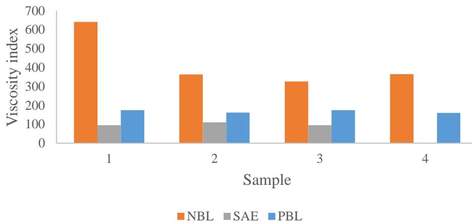
**Figure 4:** A chart of viscosity index for the biolubricant produced against SAE
