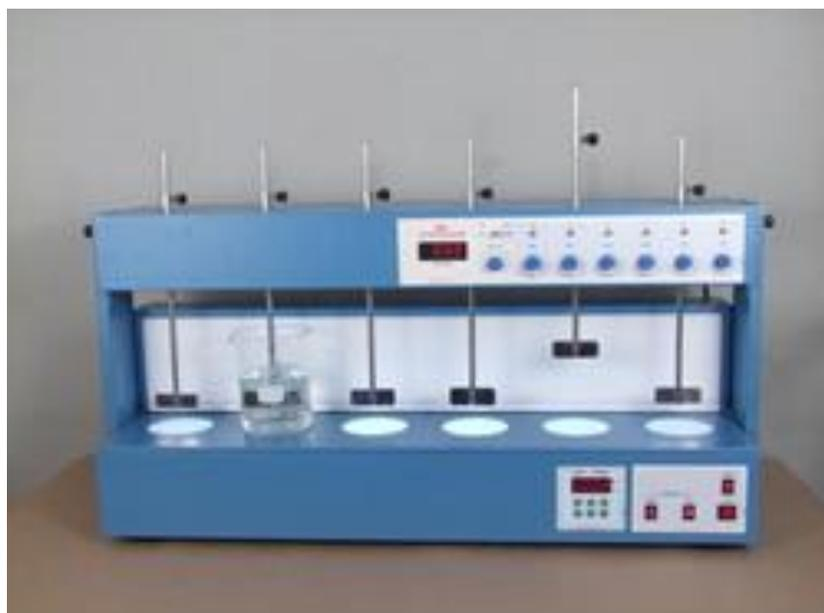
**Figure 5:** Jar Test Equipment (Flocculator)
