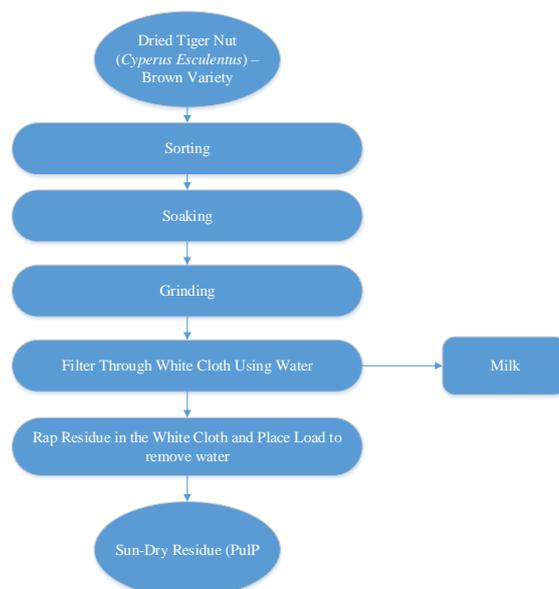
**Figure 4:** Flow Diagram for Preparation of *Cyperus esculentus* Bio-Coagulant
