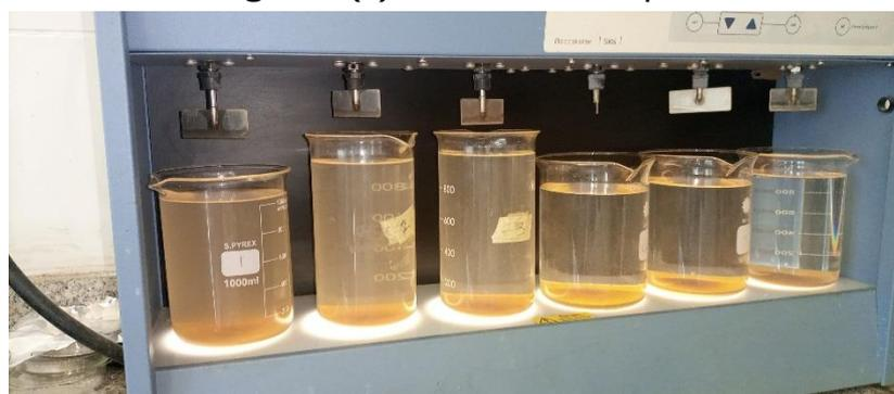
**Figure 1(b): Coagulated Water Samples**
