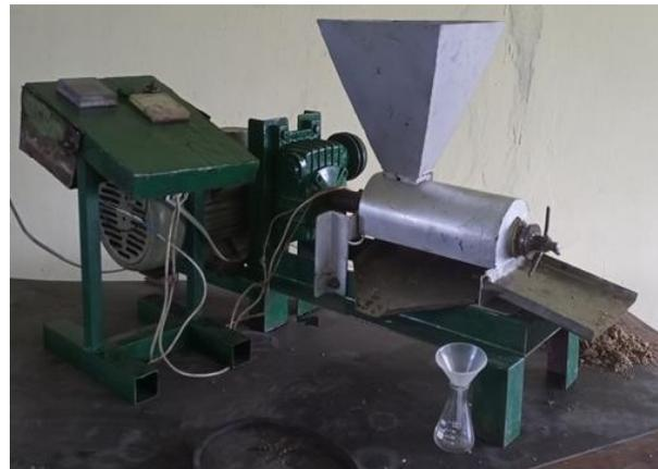
**Figure 1:** Isometric drawing of the tiger nut **Figure 2:** Pictorial view of the machine oil extraction machine
