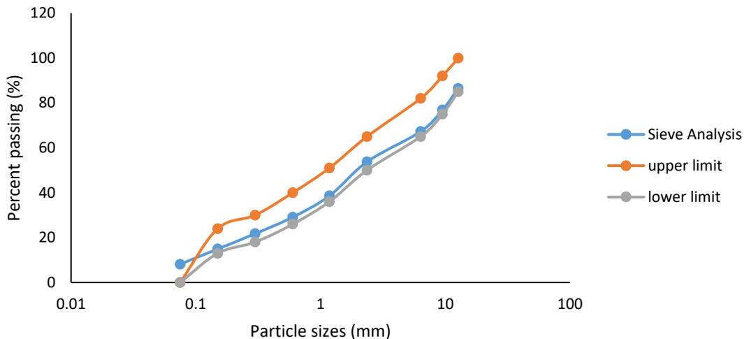
**Figure 1: Aggregate Gradation Curve**
