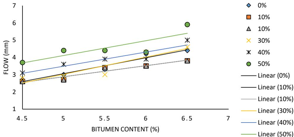
**Figure 9:** Flow versus Bitumen Content at varying CDA content.
