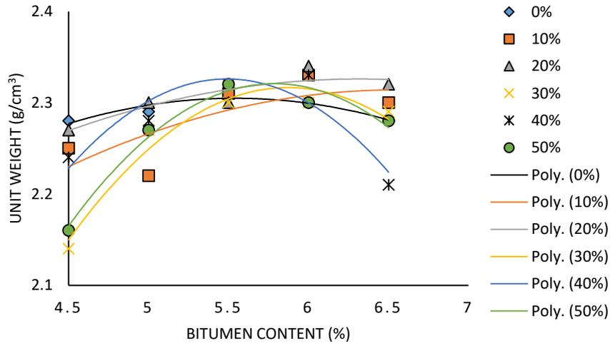
**Figure 10:** Unit Weight versus Bitumen Content at varying CDA content.
