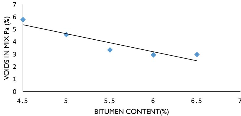
**Figure 6:** Void in Mix Versus Bitumen Content
