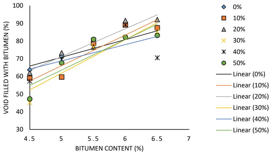
**Figure 13:** VMA versus Bitumen Content at varying CDA content.
