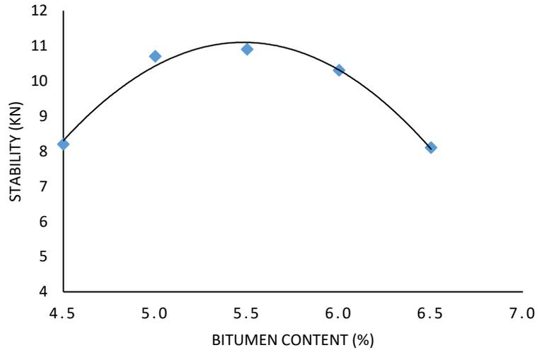
**Figure 2:** Variation of Stability with Bitumen Content
