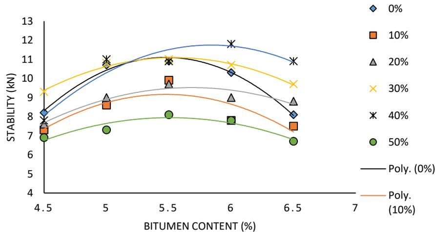
**Figure 8:** Stability Versus Bitumen Content at varying CDA content.
