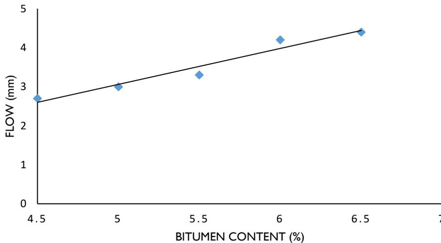
**Figure 3:** Variation of flow with Bitumen Content
