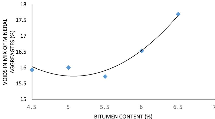
**Figure 5:** VMA versus Bitumen Content
