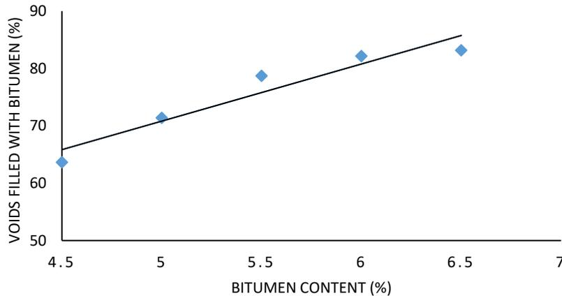
**Figure 7:** VFB versus Bitumen Content
