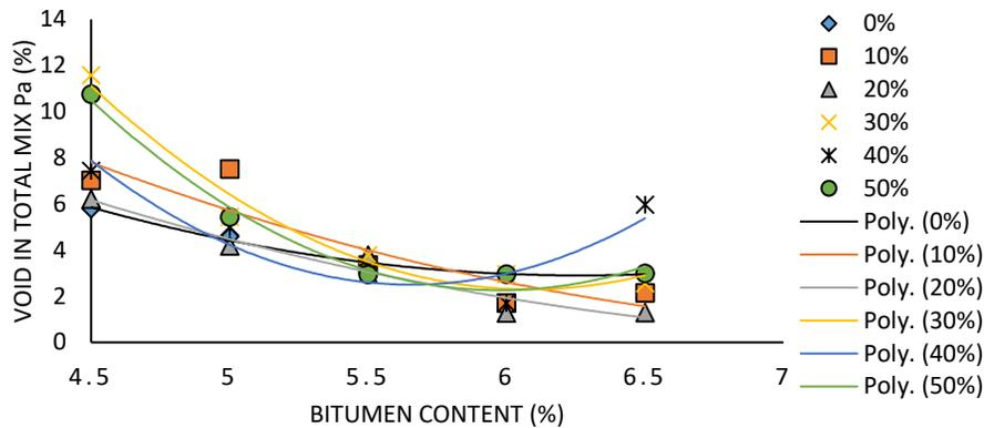
**Figure 12:** Void in Total Mix versus Bitumen Content at varying CDA content.
