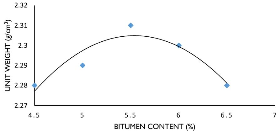
**Figure 4:** Unit Weight versus Bitumen Content
