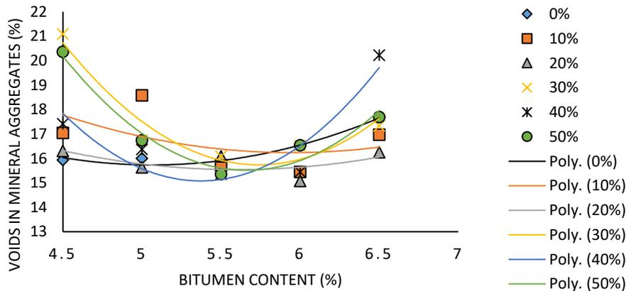
**Figure 11:** VMA versus Bitumen Content at varying CDA content.
