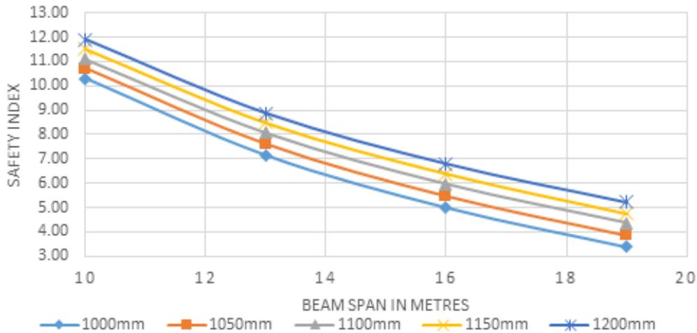
**Figure 8:** Shear safety index Vs Beam span for various beam depth for 30 N/mm<sup>2</sup> characteristic strength of concrete
