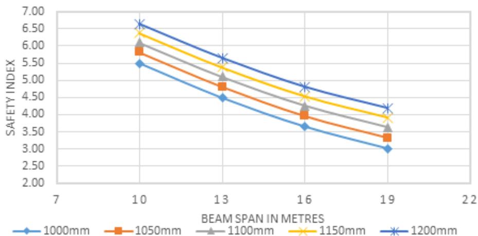
**Figure 9:** Shear safety index Vs Beam span for various beam depth for 35 N/mm<sup>2</sup> characteristic strength of concrete
