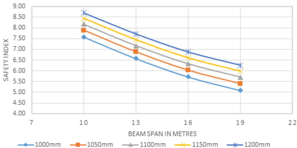
**Figure 11:** Shear safety index Vs Beam span for various beam depth for 50 N/mm<sup>2</sup> characteristic strength of concrete
