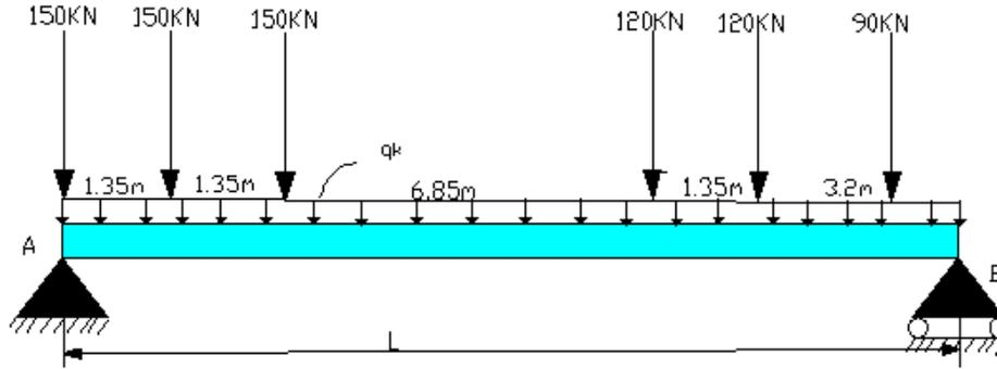
**Figure 2:** Arrangement of Load Model I for critical shear
