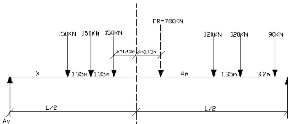
**Figure 3:** Arrangement of maximum bending of Load Model I
