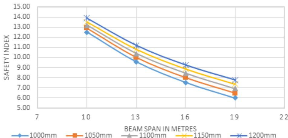
**Figure 6:** Flexural safety index Vs Beam span for various beam depth for 40 N/mm<sup>2</sup> characteristic strength of concrete
