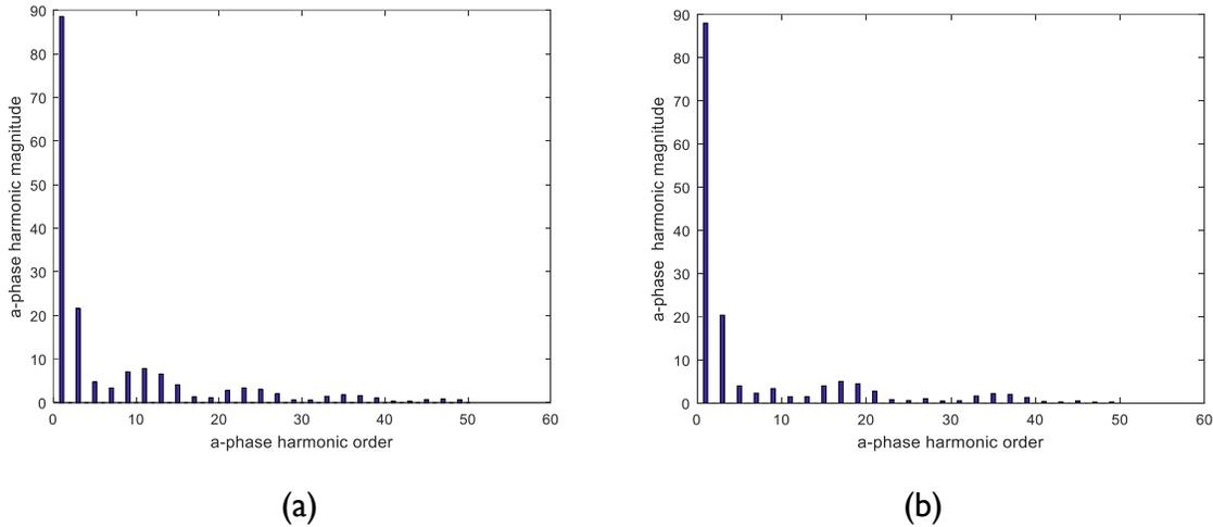
Fig. 2: Winding Function for the (a) 24-Slot Stator, and (b) 36-slot Stator
