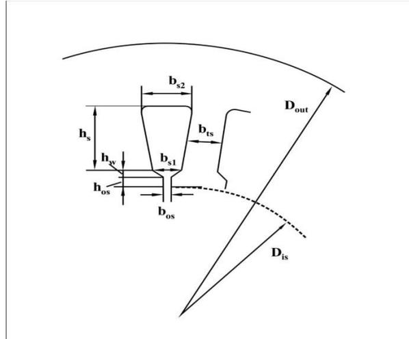
Fig. 1: The adopted Stator Slot and its parameters
