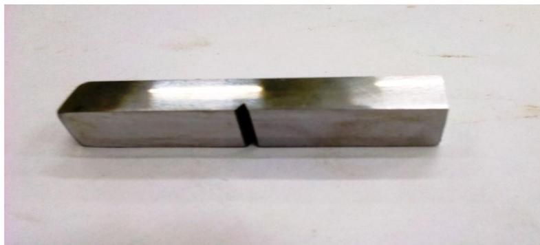
Figure 3: Charpy test specimen
