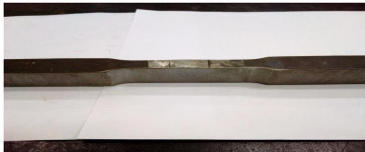
Figure 1: Tensile test specimen
