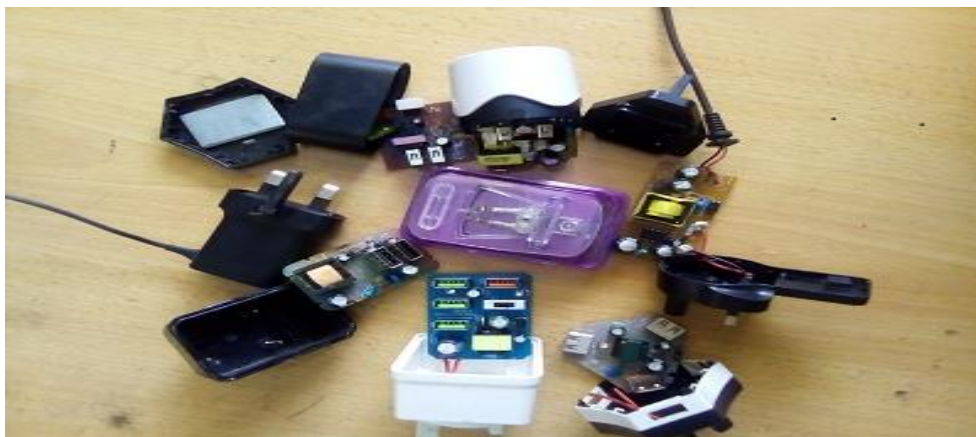
Figure 1: Sampled failed charging modules
